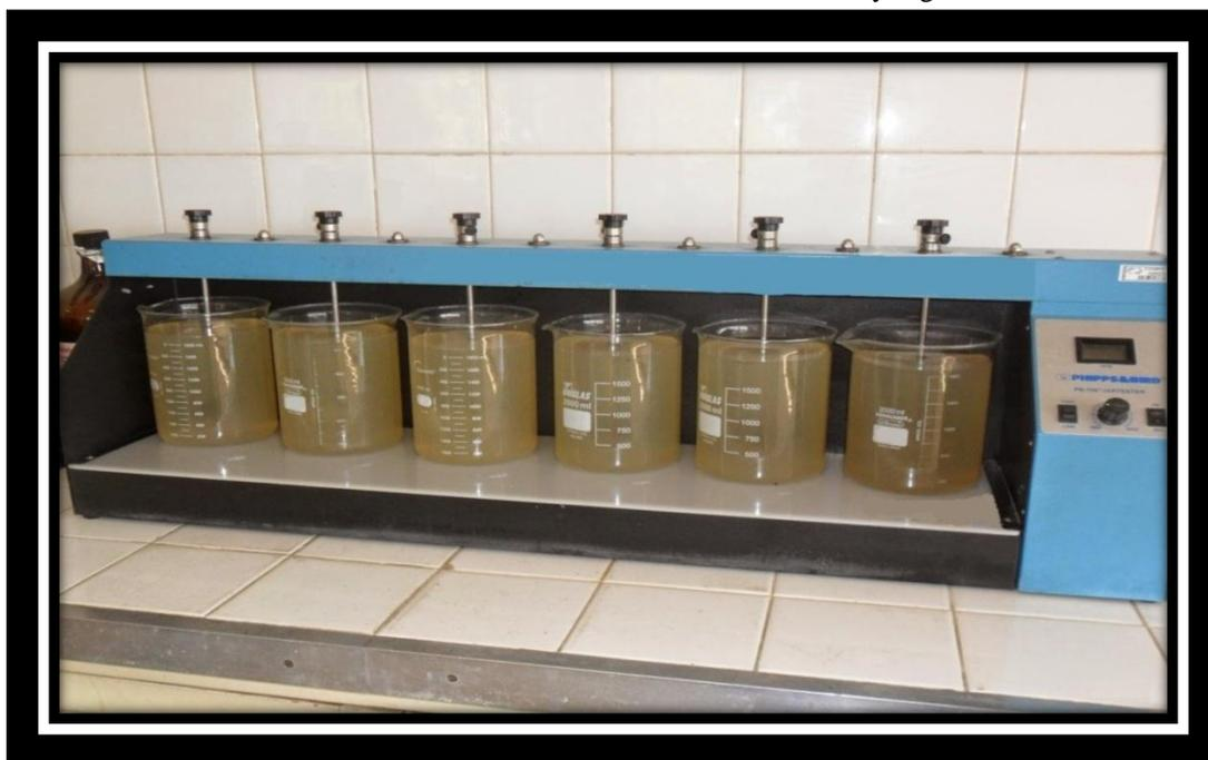
Figure 3. Jar test for turbidity river water.
