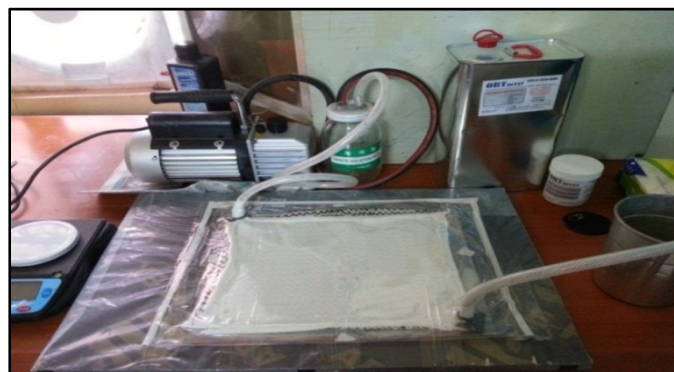
Figure (3): Vacuum bagging technique.
