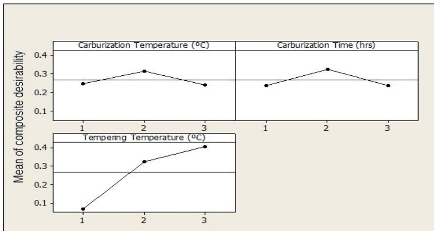
**Figure (2): Mean plot of composite desirability.**
