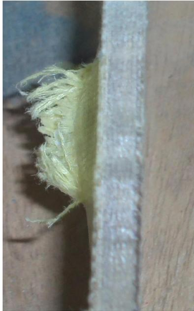
**Fig.14. A cross sectional view of perforated zone composite material target of 20 layer woven fiber Kevlar/  $\text{Al}_2\text{O}_3$  powder in a Epoxy matrix struck by a hemispherical projectile as  $V_i = 321.78$  m/s**
