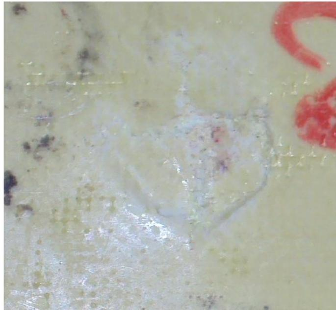
**Fig.15. Composite material target of 30 layer woven fiber Kevlar/  $\text{Al}_2\text{O}_3$  powder in a Epoxy matrix struck by a hemispherical projectile as  $V_i = 385$  m/s**
