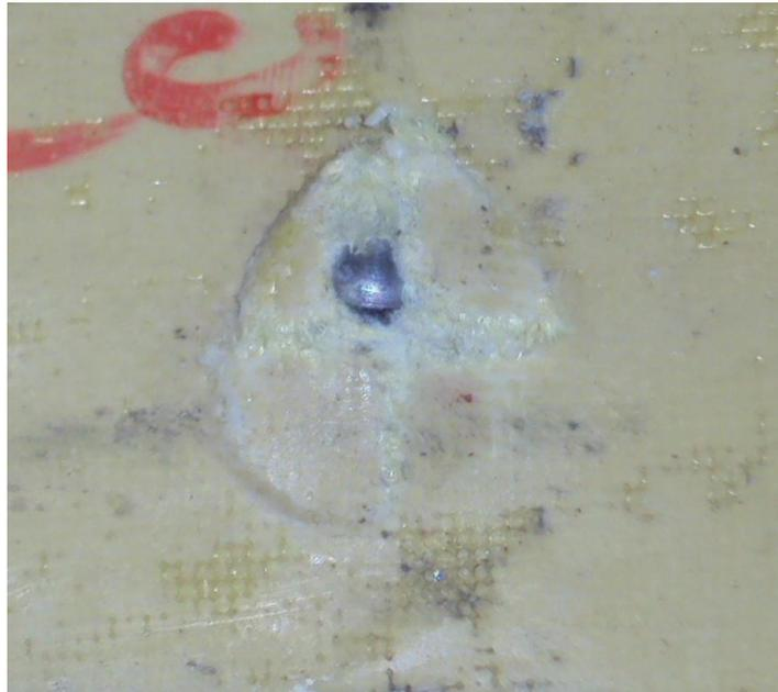
**Fig.16. Composite material target of 30 layer woven fiber Kevlar/ Al<sub>2</sub>O<sub>3</sub> powder in a Epoxy matrix struck by a hemispherical projectile as  $V_i = 390.87$  m/s**
