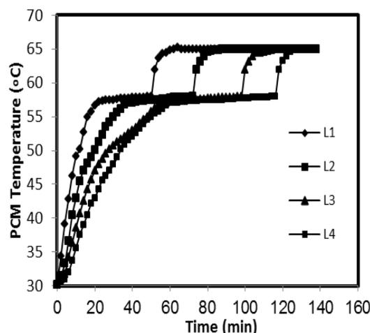
Fig. 2: Temperature History of PCM during Charging Process ( $Q= 24 \text{ L/s}$ ;  $T_{HTF}=65$ )
