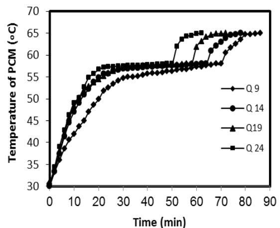
Fig. 4: Effect of HTF flow rate on charging time at L1
