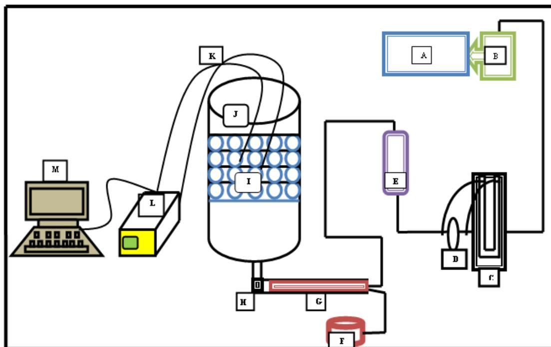
A- Air conditioning device, B- Blower, C- Manometer, D- Orifice meter, E- Rotameter, F- electric heater, G-Rode heater, H-sensor for inlet air, I- TES tank, J- spherical capsules, K- thermocouples sensor, L- data logger, M- PC
