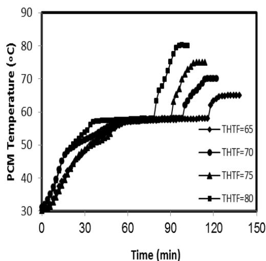
Fig. 5: Effect of Different HTF Temperatures on Charging Time at L4
