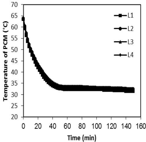
Fig. 7: Temperature History of HTF during Discharging Process ( $Q= 24$  L/s;  $T_{HTF}=65$ )
