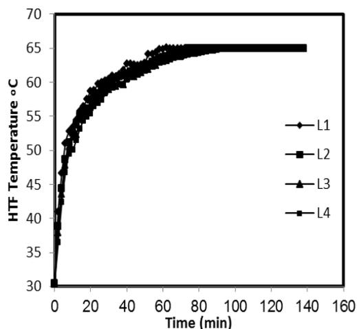
Fig. 3: Temperature History of HTF during Charging Process ( $Q=24$  L/s;  $T_{HTF}=65$ )
