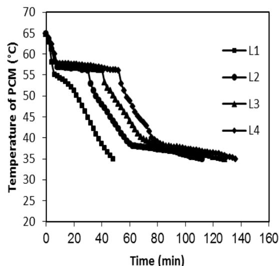
Fig. 6: Temperature History of PCM during Discharging Process ( $Q= 24$  L/s;  $T_{HTF}=65$ )
