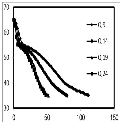
Fig. 8: Effect of HTF Flow Rate on Charging time at L1
