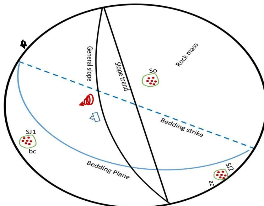
**Figure 5-** Shows the relationship among slope, bedding planes, discontinuities, and models of occur and probable failures at station No.2 in SW Haibt Sultan mountain Kalkasmag-Koysinjaq.
