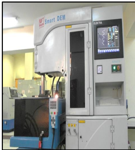
Figure (1): EL PULSE 15 Electra WED Machine being used in experimental work.
