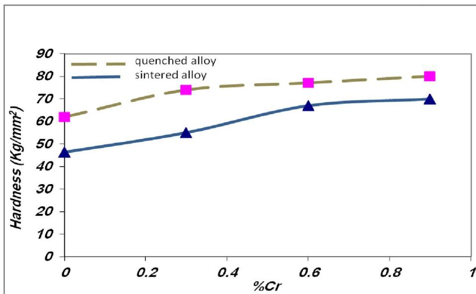
Figure (5). Hardness-%Cr relation for sintered and quenched copper base shape memory alloy.
