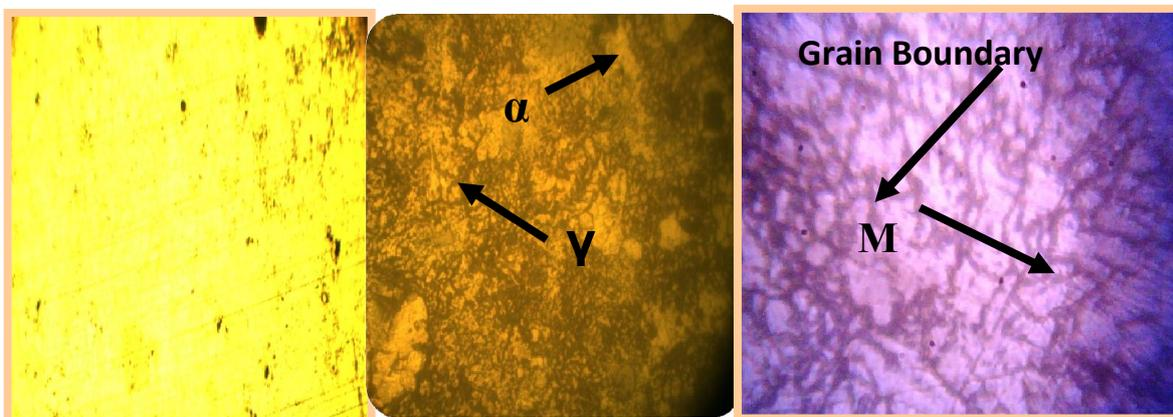
Figure(1).Microstructures for alloy(Cu-13%Al-4%Ni): a-sintered alloy not etched 40x,b-sintered alloy etched40x ,c-quenched alloy and etched 200x
