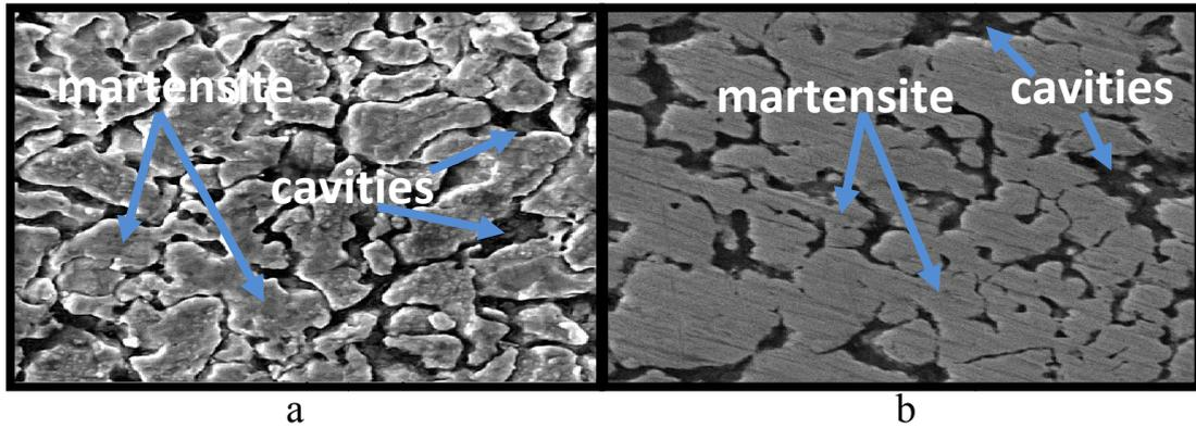
Figure(4). SEM image for etched in direct quenching state for: a- alloy (Cu-13%Al-4%Ni) b- alloy (Cu-13%Al-4%Ni-0.9Cr)
