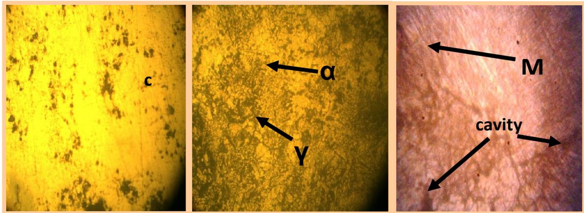
Figure(2).Microstructures for alloy(Cu-13%Al-4%Ni-0.9Cr): a-sintered alloy not etched40x b-sintered alloy etched10x ,c-quenched alloy etched 200x
