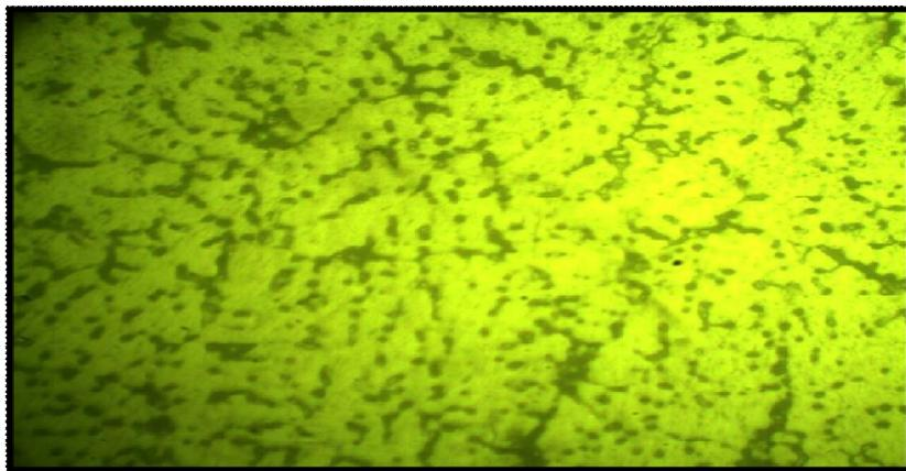
**Figure (8)** show microstructure for (Al-10%Mg) alloy (200X).
