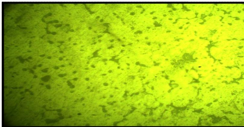
**Figure (7)** show microstructure for (Al- 5%Mg) alloy(200X).
