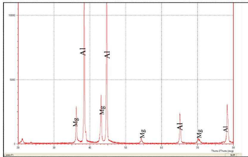
**Figure (5)** represent the diffraction of x-ray of Al- 15% Mg alloy.
