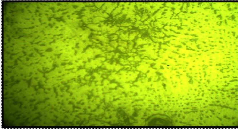
**Figure (9)** show microstructure for (Al-15%Mg) alloy (200X).
