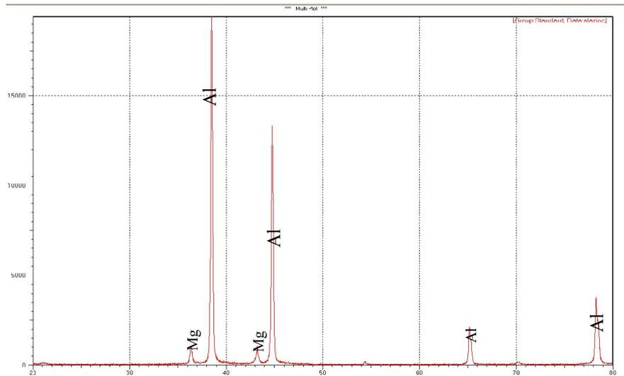
**Figure (3)** represent the diffraction of x-ray of Al- 5 % Mg alloy
