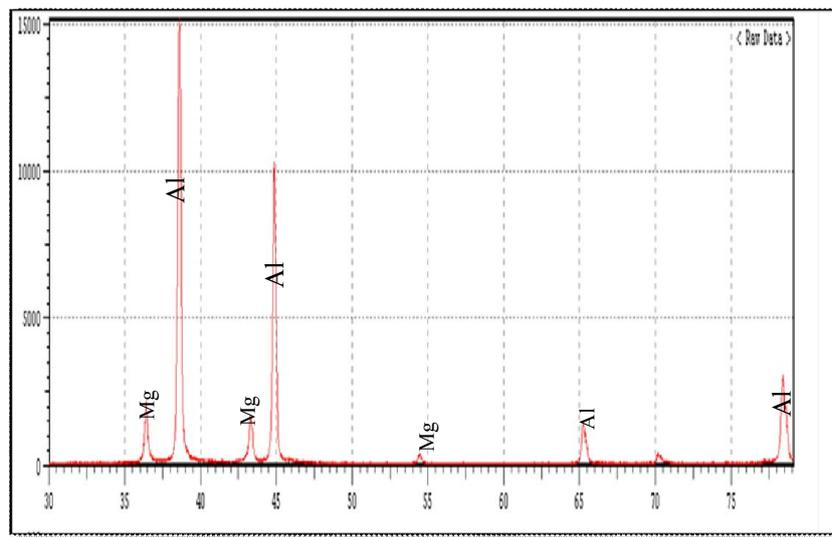
**Figure (4)** represent the diffraction of x-ray of Al- 10% Mg alloy.
