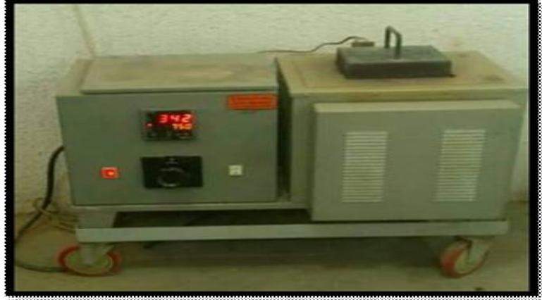
Figure (1) show melting furnace.
