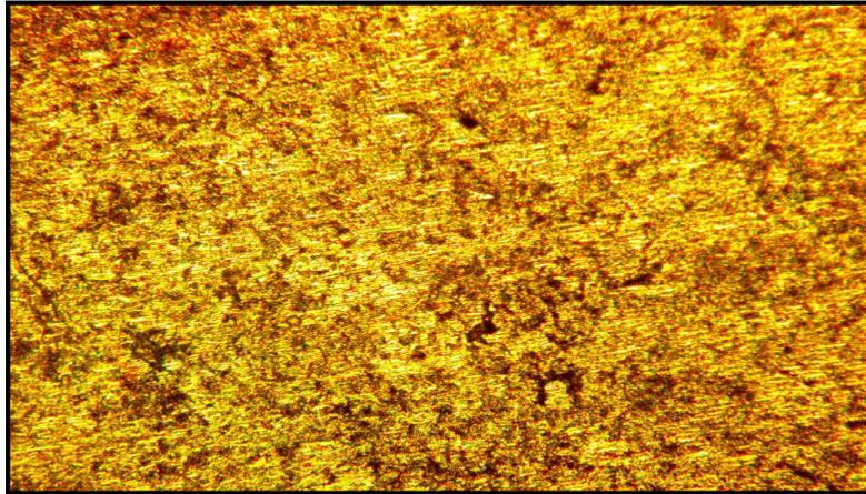
**Figure (6)** show microstructure for pure aluminum (200X).
