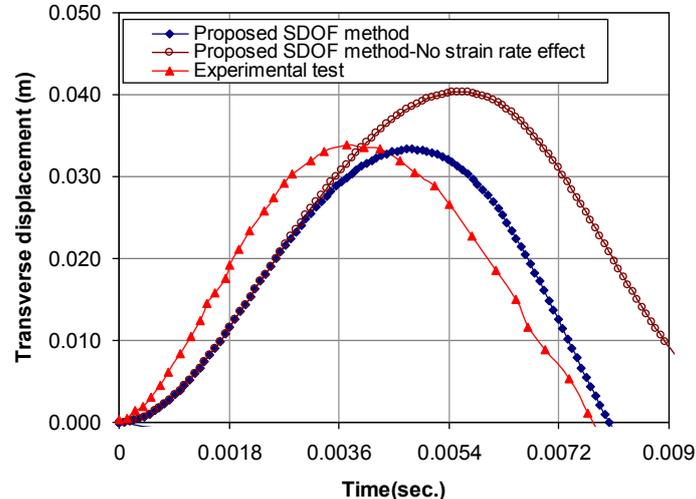
**Figure 13: Comparison of the transverse mid span displacement time history of the tested case No.3 between the proposed equations (with and without the inclusion of the strain rate effects) and the experimental test results (Nassret. al, 2012)**
