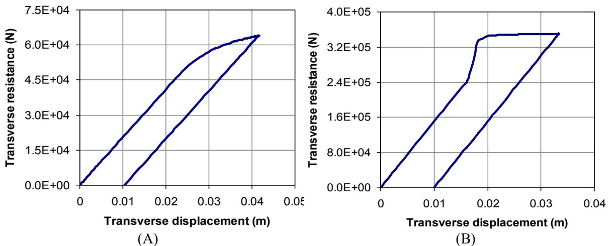
**Figure 12:** Resistance function-mid span displacement behavior of the steel beam.(A) test case 2;(B) test case 3
