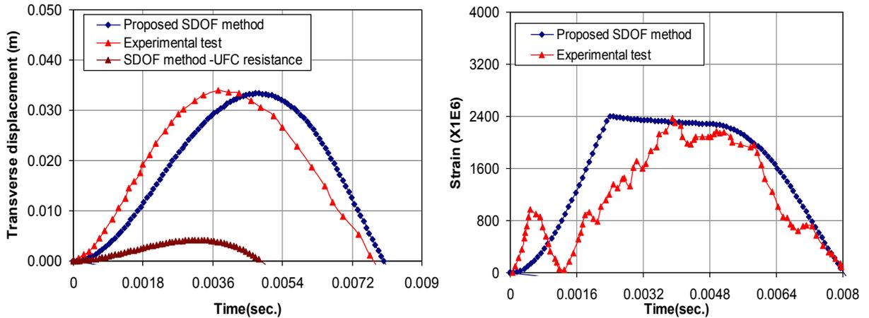
**Figure 11** Comparison between the proposed SDOF method and the experimental test results of the test case No.3(Nassr *et. al.*, 2012,Nassr., 2012)
