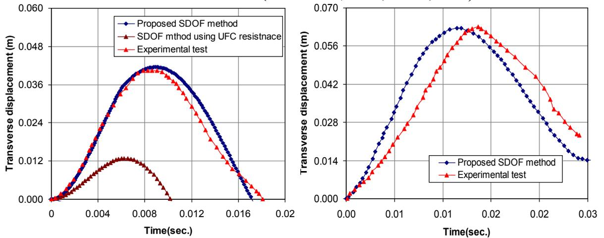
Figure 10: Comparison between the proposed SDOF method and the experimental test results of the test case No. 2 (A) and test case No. 5 (Nassr *et. Al*, 2012, Nassr., 2012)
