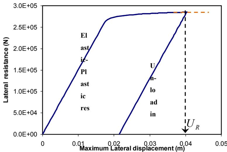
Figure 7: Generalized non-linear resistance-displacement relationship of steel beams
