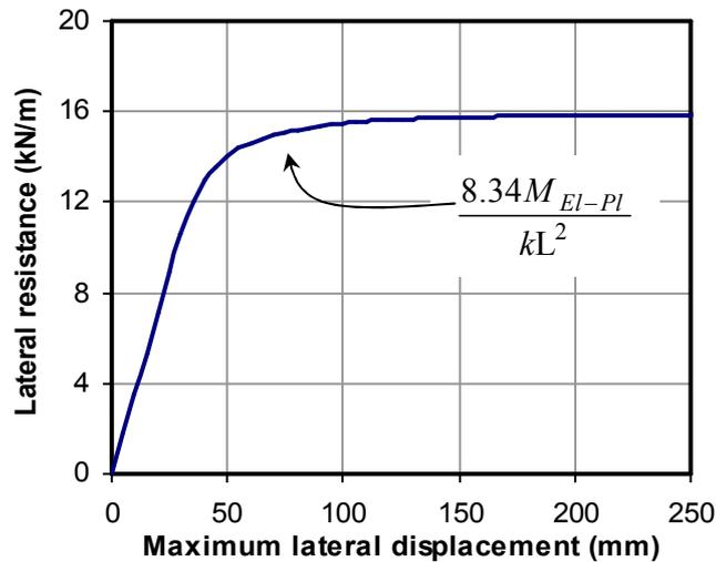
Figure 5: Nonlinear elastic-plastic behavior of the resistance function of a simply supported beam
