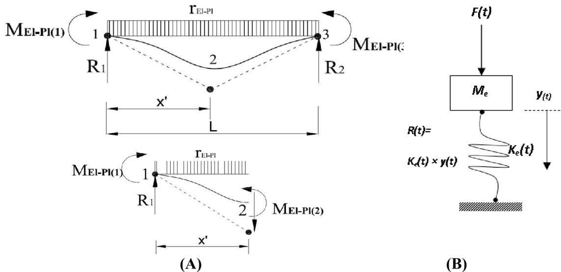
Figure 1: Steel beam model (A) with the equivalent SDOF model (B)
