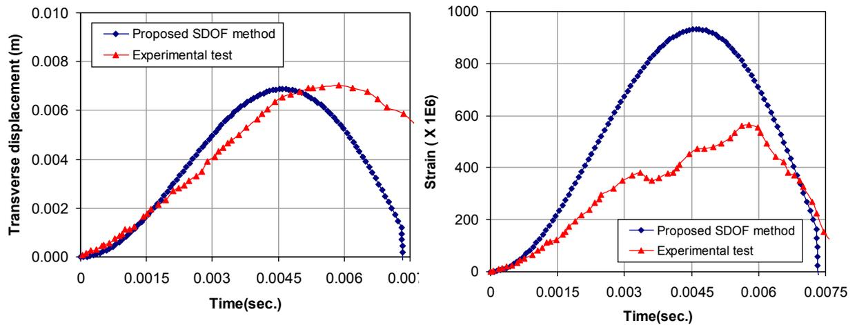
Figure 9: Comparison between the proposed SDOF method and the experimental test results of the test case No.1 (Nassr *et. al*, 2012, Nassr., 2012)
