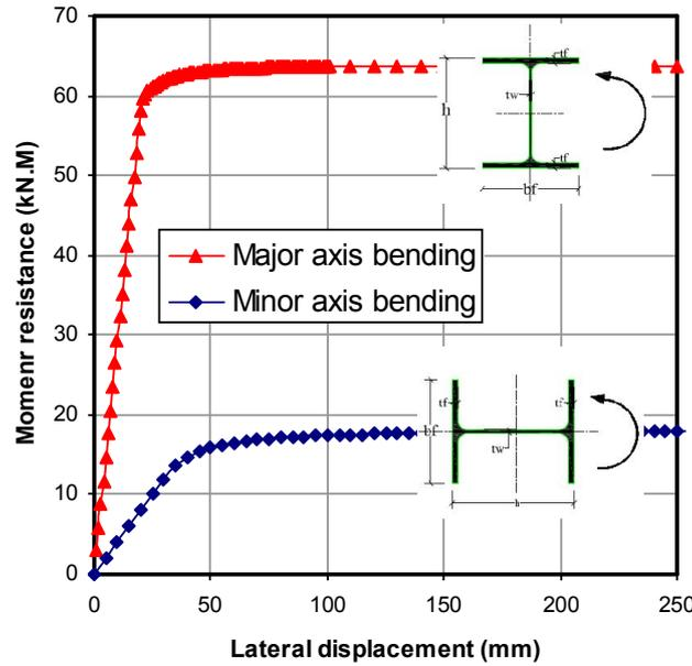
**Figure 4: Elastic Plastic moment –displacement relationship of steel beams sections bent about major and minor axes.**
