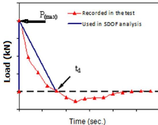
Figure 6: The idealized blast load-time function used in the equivalent SDOF model
