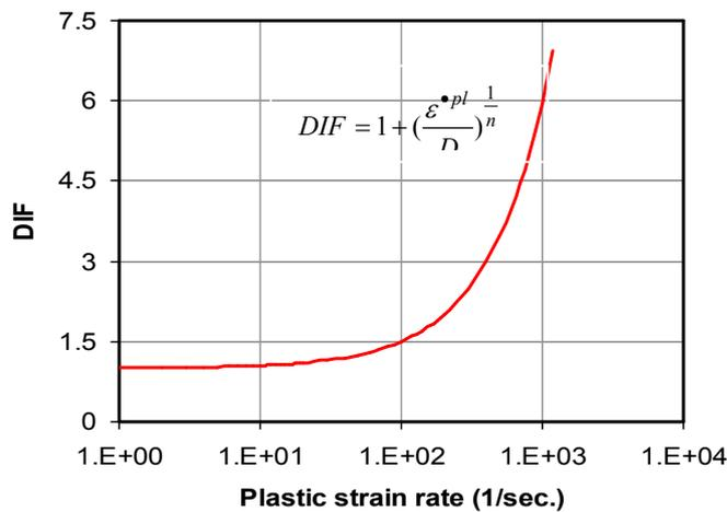
**Figure 8: Dynamic amplification factor (DIF) as a function of the plastic strain rate ( $\dot{\varepsilon}^{pl}$ )**
