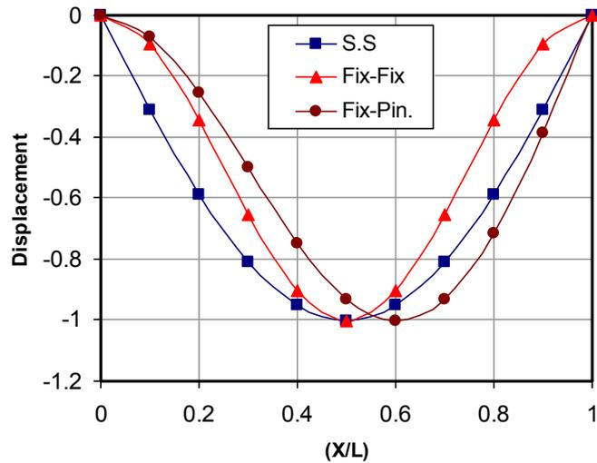
**Figure 3: Assumed displacement shapes of steel beams for three cases of boundary conditions**
