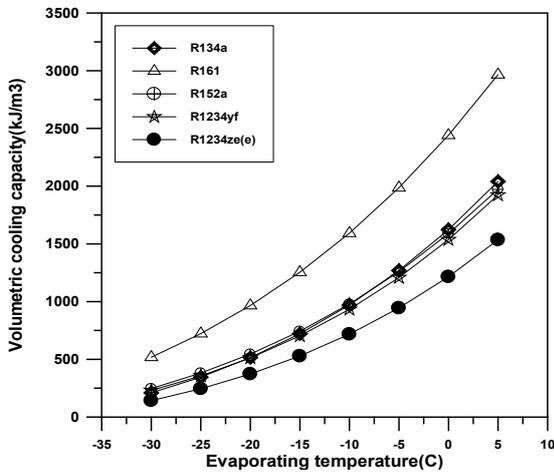
Fig. 5 shows volumetric cooling capacity versus evaporating temperature
