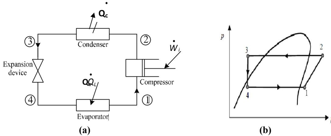
**Fig. 2: a) System schematic diagram b) Pressure-enthalpy diagram of a simple refrigeration cycle**
