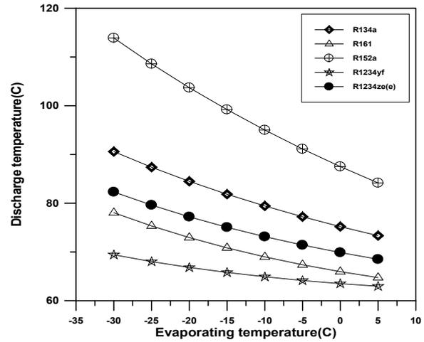
Fig. 10 6 shows compressor discharge temperature versus evaporating temperature
