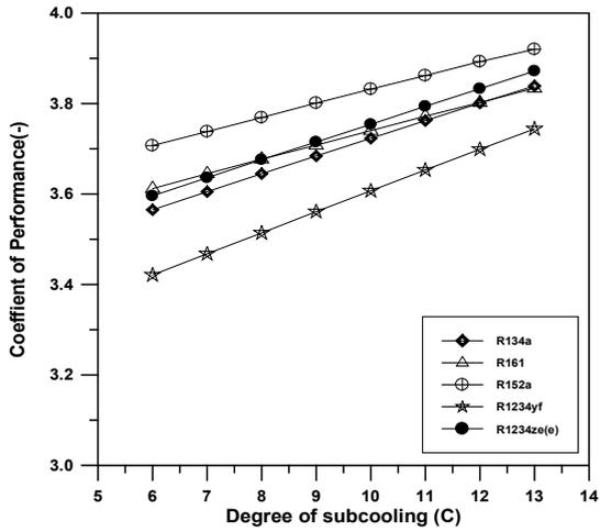
Fig. 3 shows COP versus sub-cooling temperature
