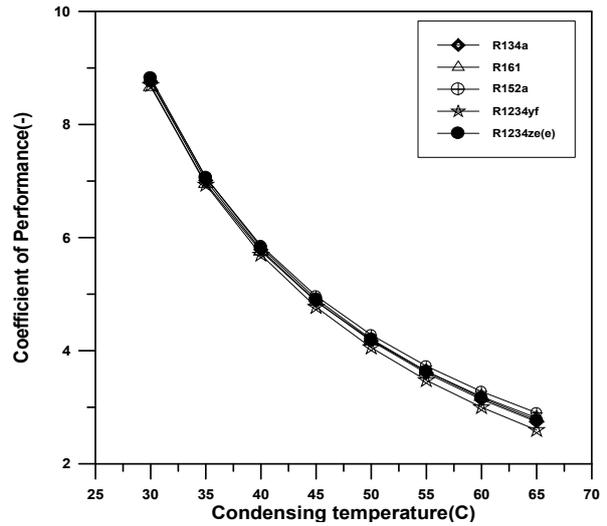
Fig. 16 shows COP versus condensing temperature
