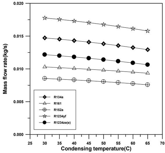
Fig. 15 shows refrigerant mass flow rate versus condensing temperature
