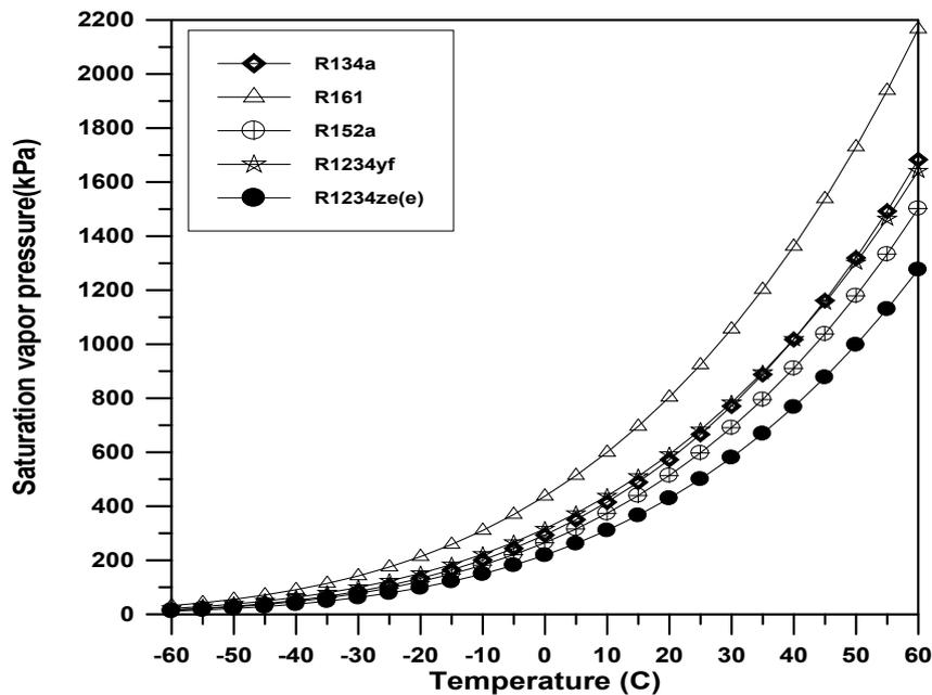
Fig. 1: Saturation pressure versus temperature
