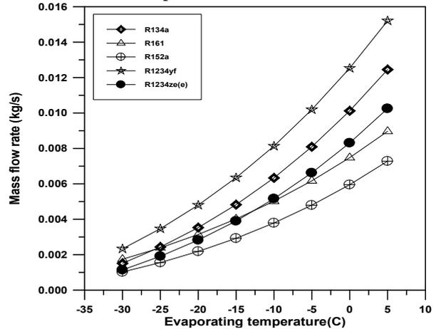
Fig. 8 refrigerant mass flow rate versus evaporating temperature
