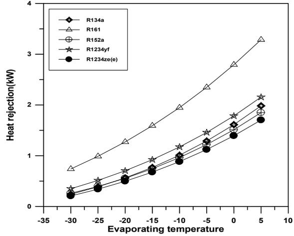
Fig. 6 shows heat rejection versus evaporating temperature
