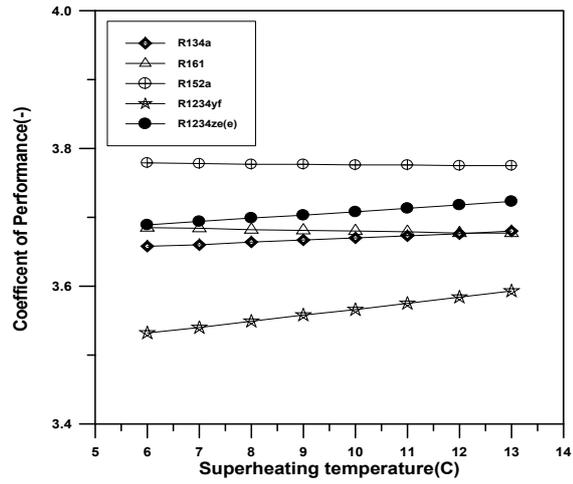
Fig. 4 shows COP versus superheating temperature
