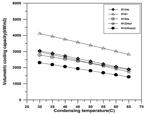
Fig. 12 6 shows volumetric cooling capacity versus condensing temperature
