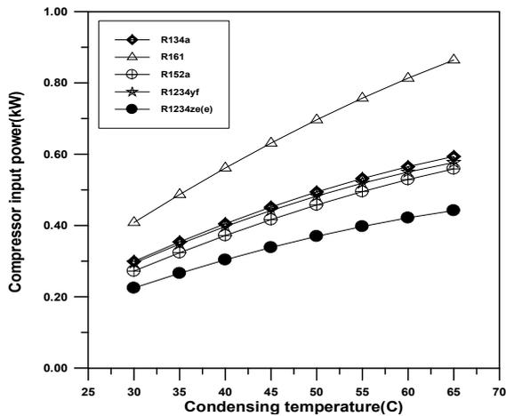
Fig. 13 shows compressor input power versus condensing temperature
