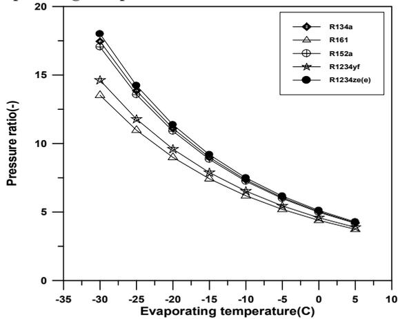
Fig. 7 shows pressure ratio versus evaporating temperature
