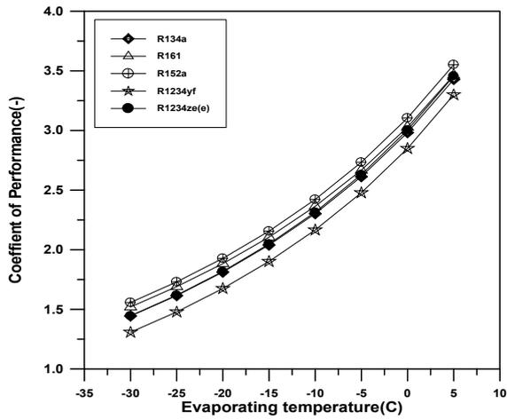
Fig. 9 6 shows COP versus evaporating temperature
