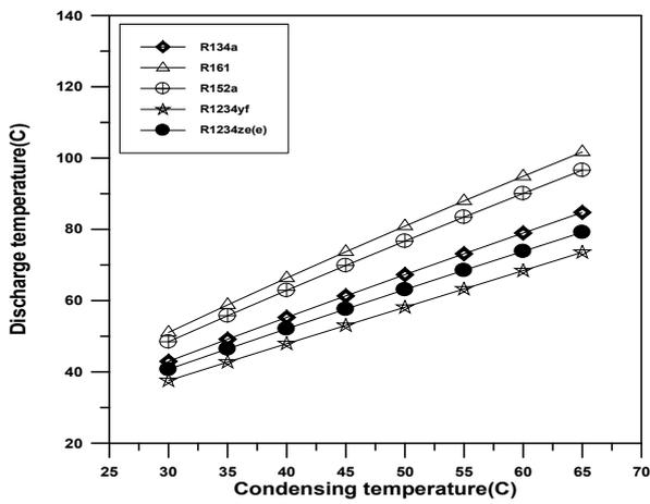
Fig. 17 shows compressor discharge temperature versus condensing temperature
