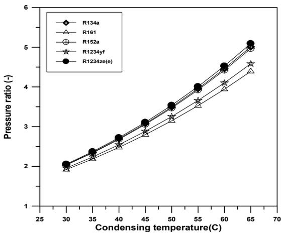
Fig. 11 6 shows pressure ratio versus condensing temperature
