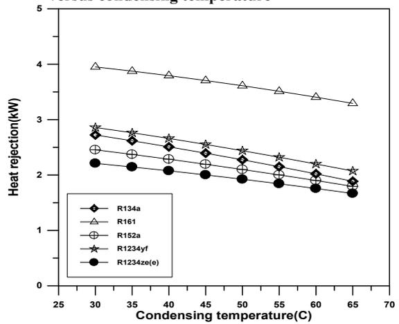
Fig. 14 shows heat rejection versus condensing temperature
