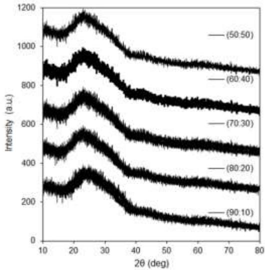
Fig. (4) The XRD patterns of the SiO<sub>2</sub> nanostructures prepared in this work using different mixing ratios of Ar:O<sub>2</sub> gases
