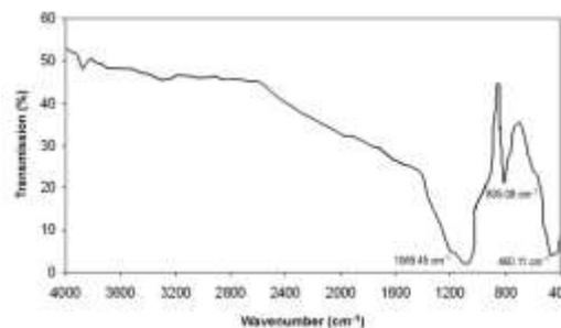
Fig. (2) The transmission FTIR spectrum of the prepared sample
