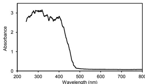
Fig. (3) The absorption spectrum of the prepared sample in the UV and visible regions (200-800nm)
