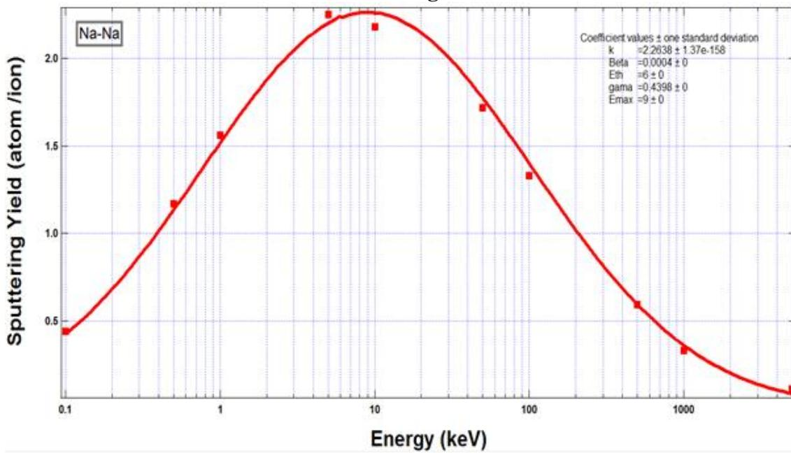
**Figure( 5): Sputtering yield vs. ion energy for sputtering of Na with theoretical equation fitting.**
