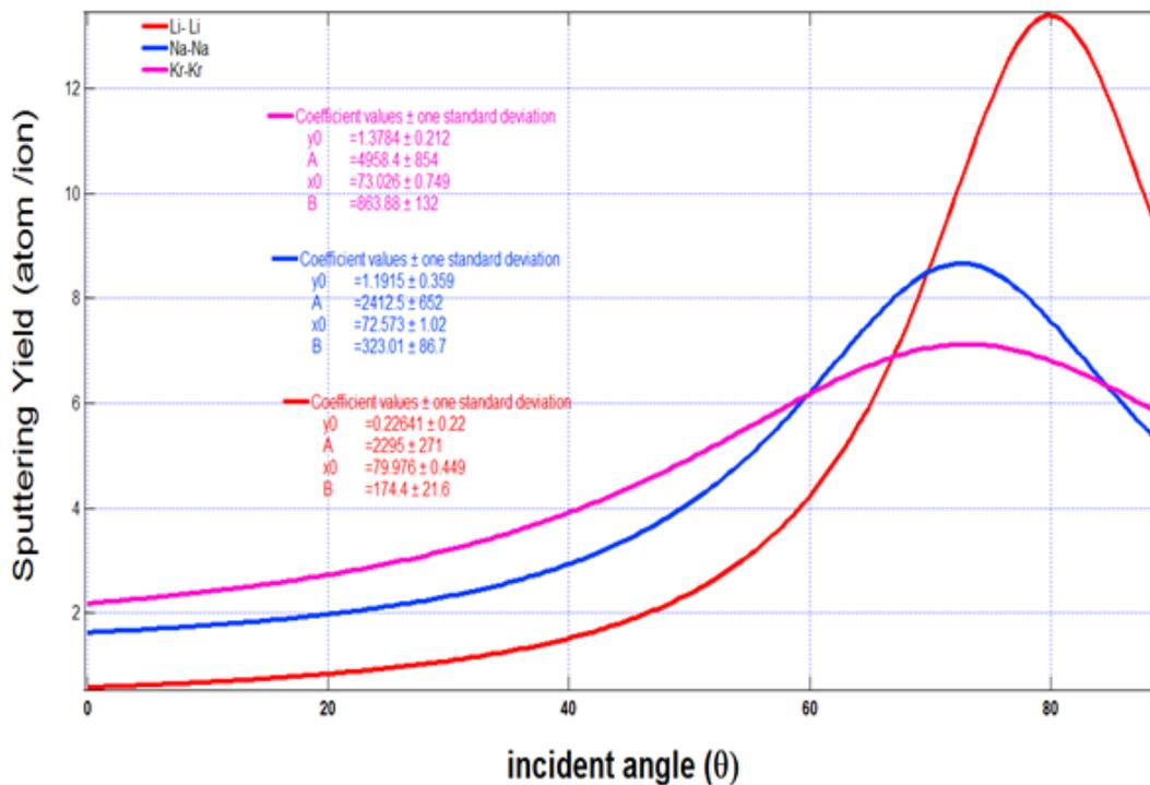
Figure( 7): The angular dependent of the sputtering yield of Li,Na and Kr with fixed ion number, the width of the target and ions energy.
