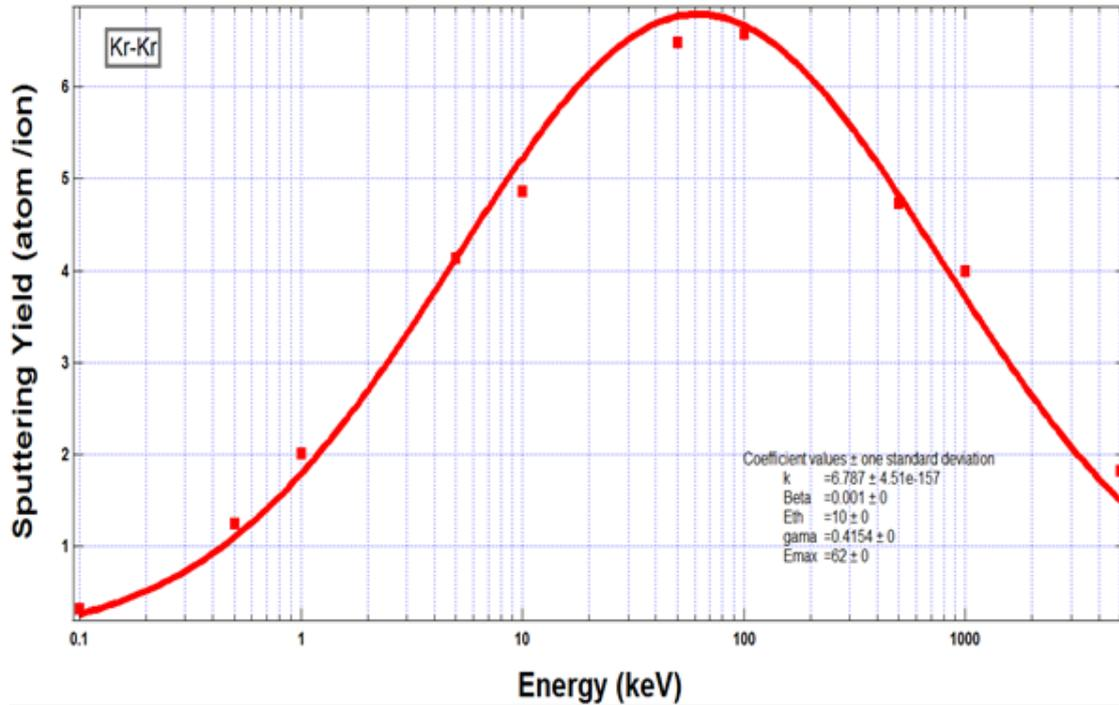
Figure (6): Sputtering yield vs. ion energy for sputtering of Kr with theoretical equation fitting.
