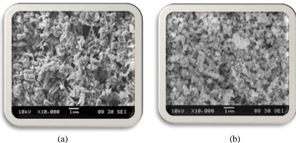
**Figure 2:** SEM images in top view of (a) porous silicon (b) oxidation porous silicon.
