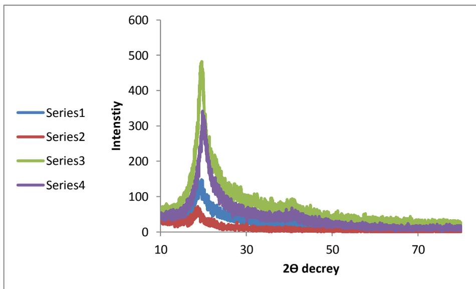
Fig (1) X-ray diffraction of PVA films for different thickness.
