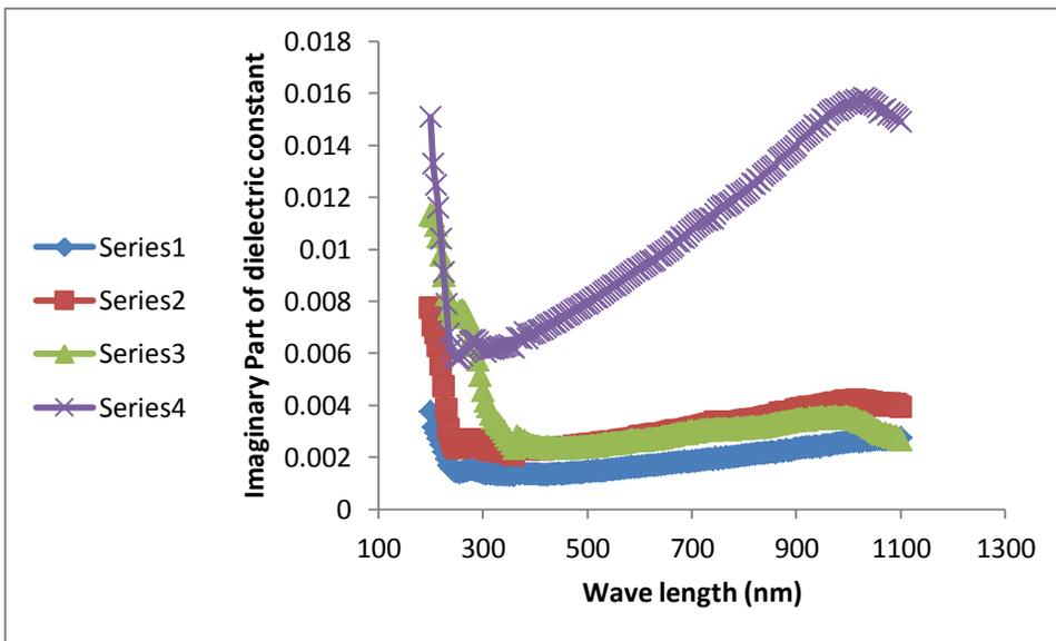
Fig.(7) Imaginary part Dielectric constant of PVA versus wavelength for different thickness films.
