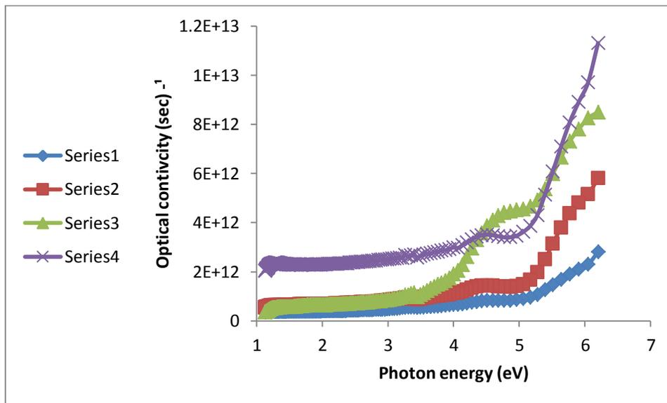
Fig.(8)Optical Conductivity of PVA versus Photon energy for different thickness films.
