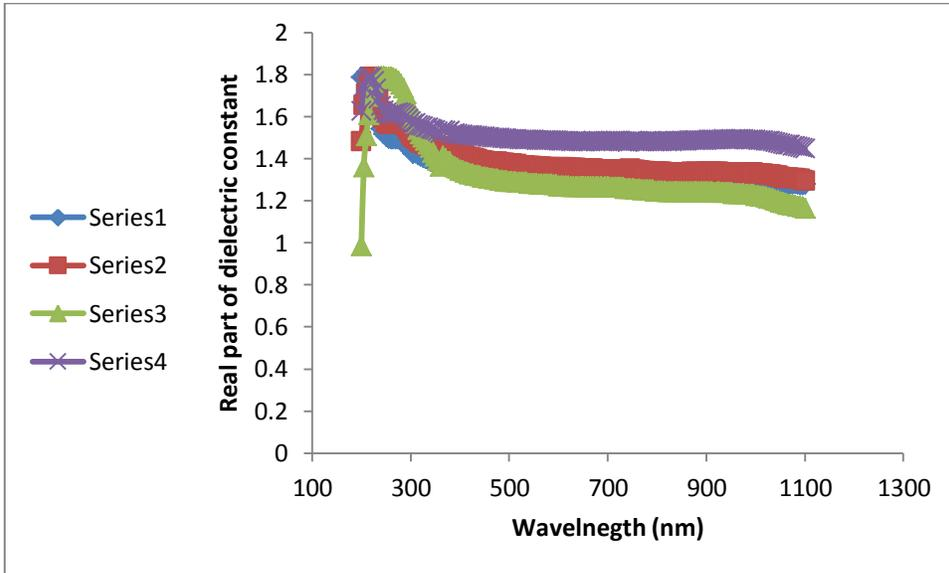
Fig. (6) Real part of Dielectric Constant of PVA films versus wavelength for different thickness films.
