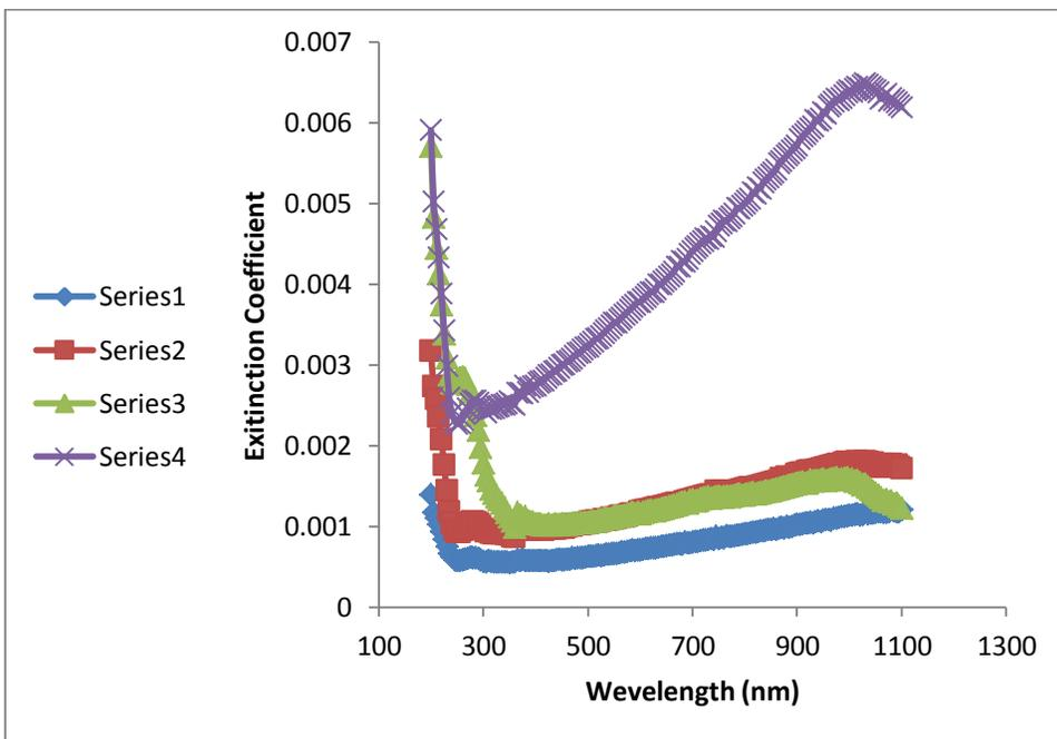
Fig. (5) Extinction coefficient versus wavelength for as deposited films.
