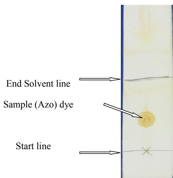
**Figure(1) :Thin layer chromatography of prepared azo dye**
