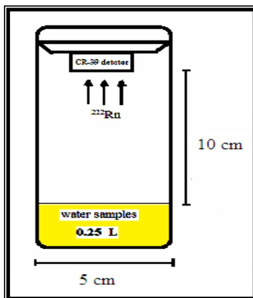
Figure (1) A schematic diagram of the sealed-cup technique in drinking water samples.
