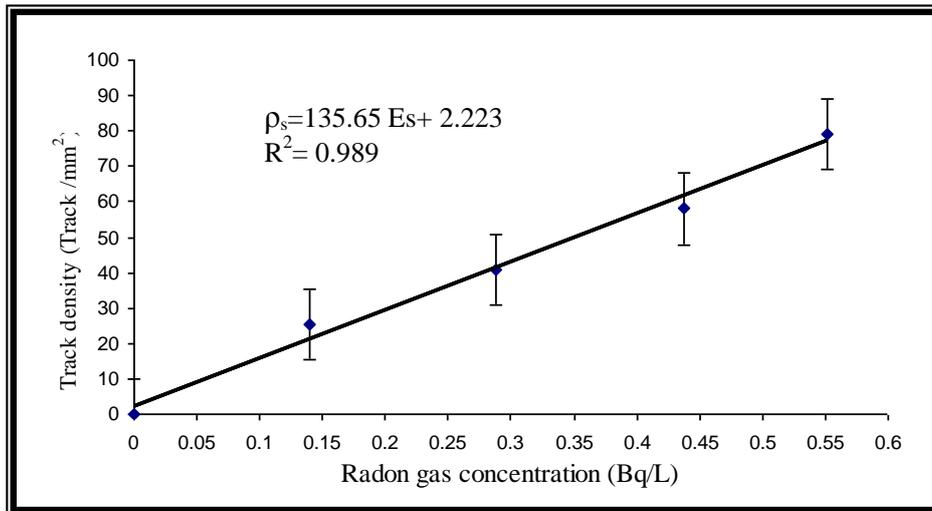
Figure (2) the relation of radon gas concentration and track density in water standard samples.
