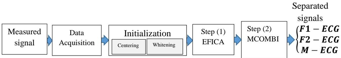
**Figure 5: Block diagram of the proposed algorithm**
