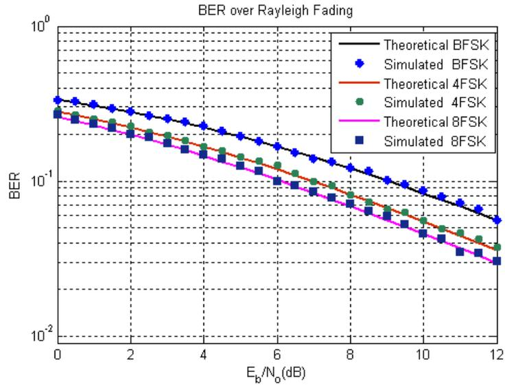
**Figure 5. Comparison of simulated and theoretical BER, M=2, 4, 8 for Rayleigh channel**
