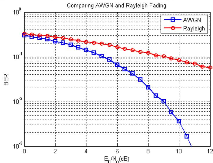
**Figure 8. Comparison of BER over AWGN and Rayleigh channel**
