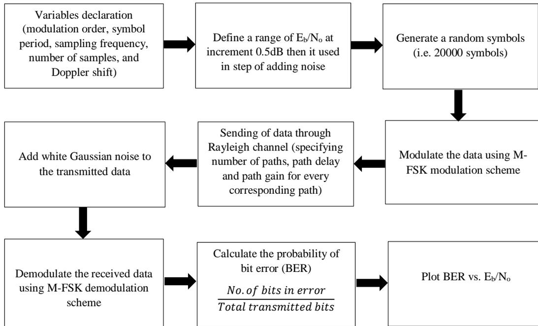
Figure 3. Block diagram of simulation process
