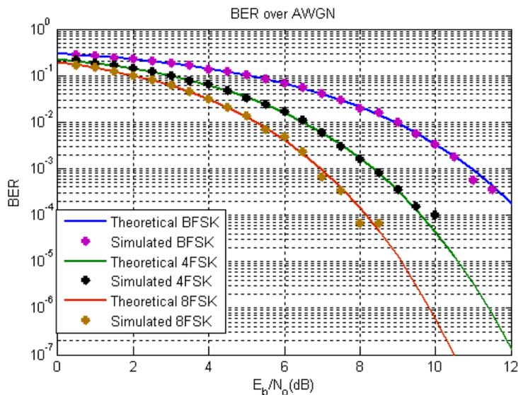
Figure 4. Comparison of simulated and theoretical BER,  $M=2, 4, 8$  for AWGN channel
