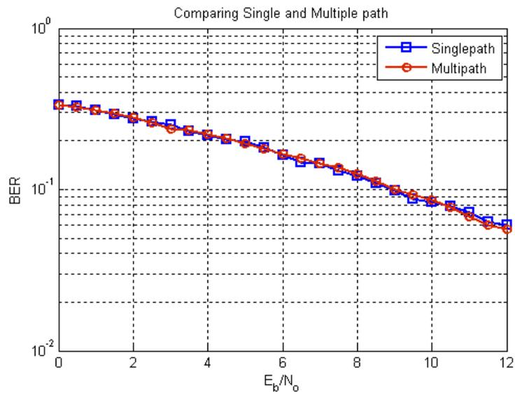
**Figure 6. Comparison of single and multiple path of BER for Rayleigh channel**
