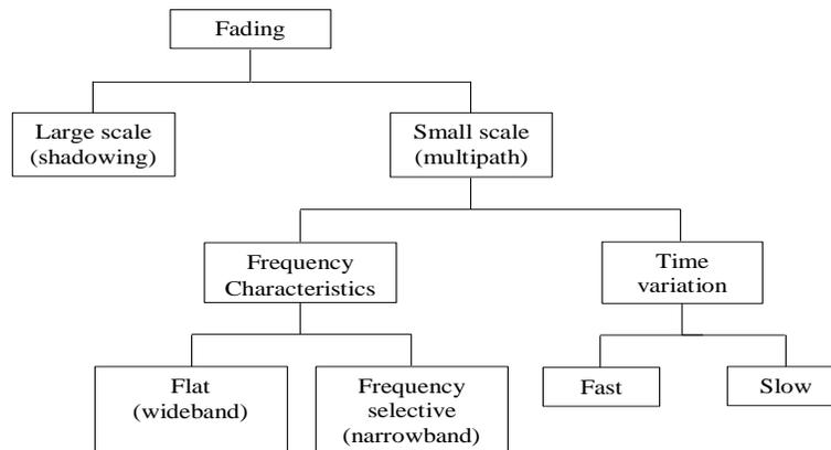
Figure 1. Block diagram summarizing the different types of fading
