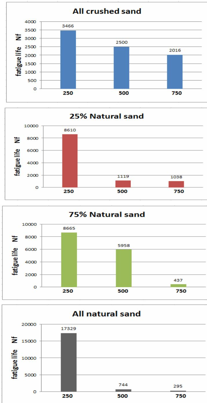
Figure (1): Effect of natural sand on fatigue life at (250, 500 and 750) microstrain
