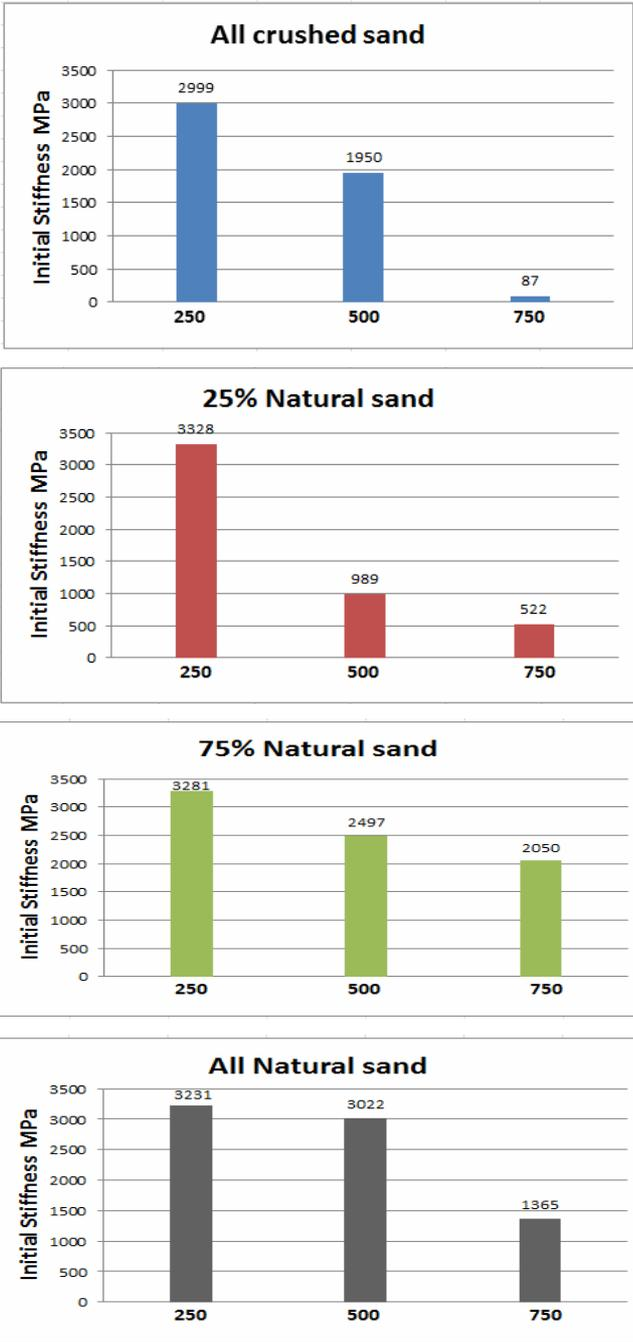
Figure (2):Effect of natural sand on initial stiffness at (250, 500 and 750) microstrain
