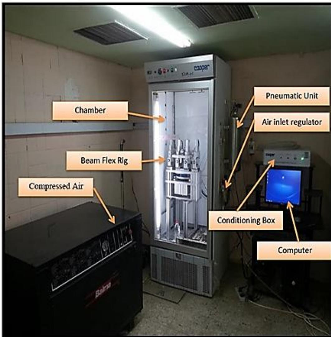
**Plate (2): Four Point Bending Beam device and Testing Equipment**
