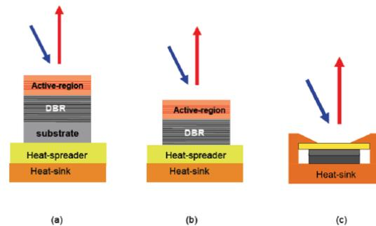
Fig. (5) VECSEL structure designs for thermal management
