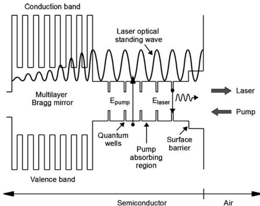
Fig. (2) Operating principles of optically pumped vertical external cavity surface emitting lasers (VECSELs) [4]
