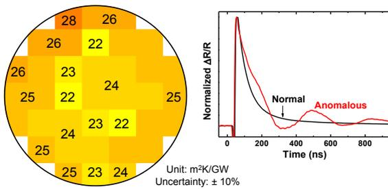
Fig. (5) Three-inch GaN-on-MW diamond wafer and its  $TBR_{eff}$  map. Representative thermoreflectance transients are shown corresponding to normal regions and a local imperfection (data from a different wafer, for illustration only), respectively
