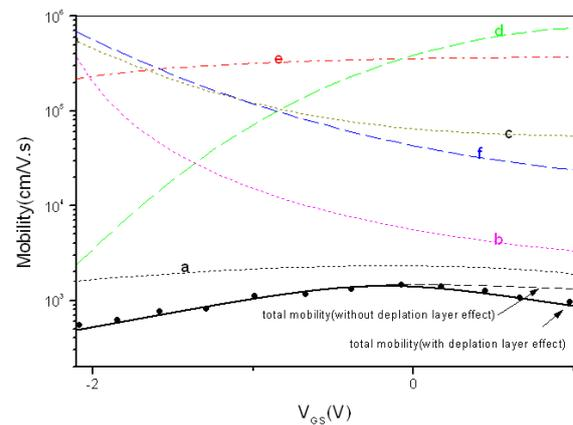
Fig. (6) Total mobility versus gate source bias at 300 K for Al<sub>0.15</sub>Ga<sub>0.85</sub>N/GaN based HEMT in comparison with existence experimental data (circles) from Ref. [4]. The different scattering mechanism in the figure labeled as (a) polar optical phonon, (b) interface roughness, (c) acoustic phonon (deformation potential and piezoelectric), (d) dislocation, (e) residual impurity and (f) alloy disorder respectively
