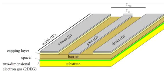
**Fig. (1) Cross section of a GaAs/AlGaAs/InGaAs pHEMT**
