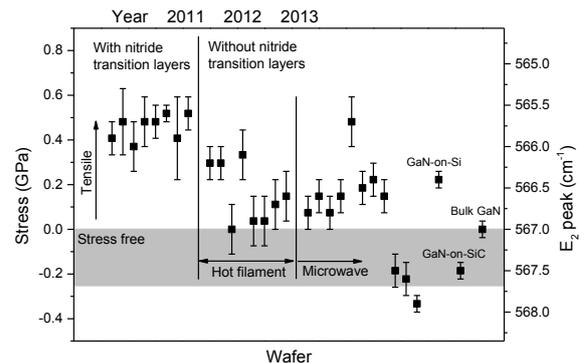
Fig. (3) The stress in the GaN layer determined by the Raman  $E_2$  peak for various GaN-on-diamond wafers through successive generations of development. The grey area indicates  $E_2$  peak positions in stress-free GaN from literature
