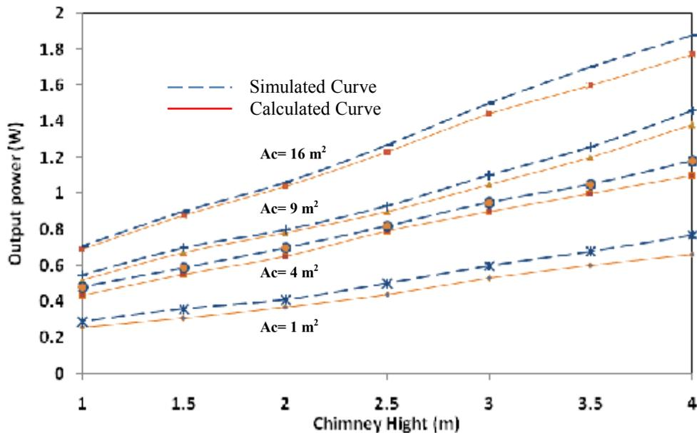
(Figure 3) Variation of the calculation and simulation output power with the variation of chimney height(m) for different collector areas  $A_c \text{ (m}^2\text{)}$ , and ambient temperature  $T_\infty = 25^\circ\text{C}$
