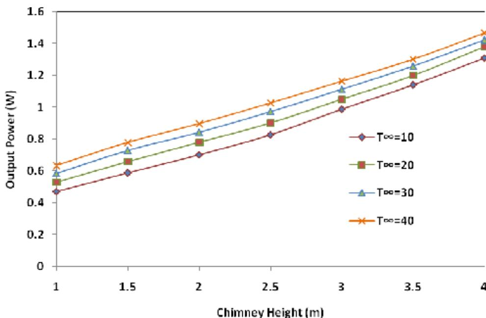
(Figure 4) Variation of output power (W) with the variation of chimney height and for different ambient temperature ( $T_{\infty}$  C<sup>0</sup>), and collector area of 9 m<sup>2</sup>.
