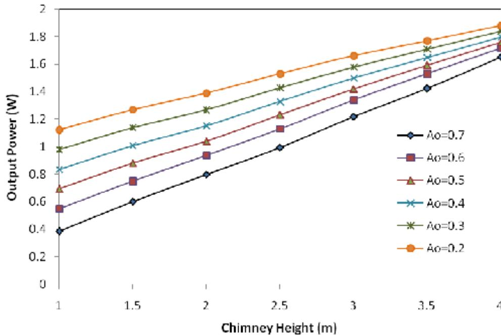
(Figure 6) Output power against chimney height for different exit area, and the collector area is 16m<sup>2</sup>.
