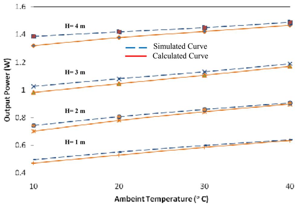
(Figure 5) Comparison between calculated and simulated output power for different ambient temperature  $T_{\infty}$  (C<sup>0</sup>) for different chimney height H (m).
