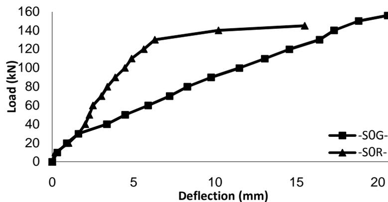
Figure (8): Load-deflection curves of beams with stirrups.
