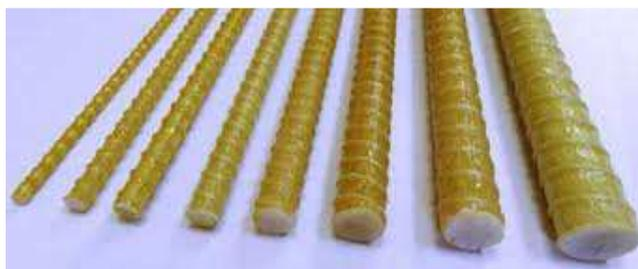
Figure1. Samples of the used GFRP bars
