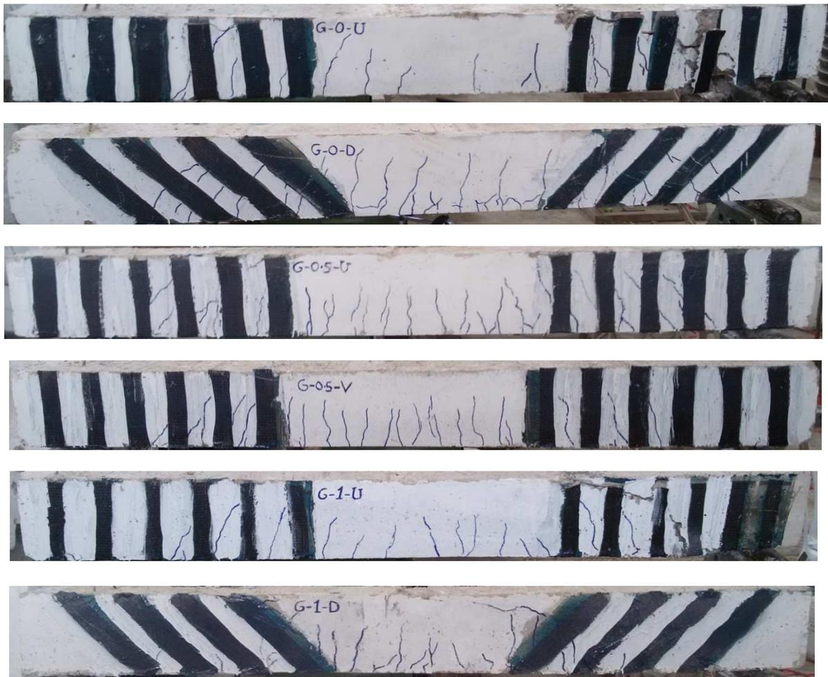
Figure (14): Cracking patterns of the tested beams.
