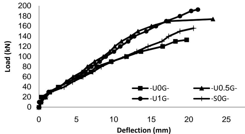
Figure (12): Load-deflection curves of GFRP reinforced beams strengthened by U-strips.
