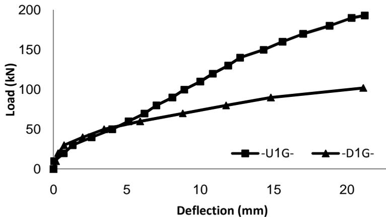
Figure (11): Load-deflection curves of GFRP reinforced beams with 1% steel fiber.
