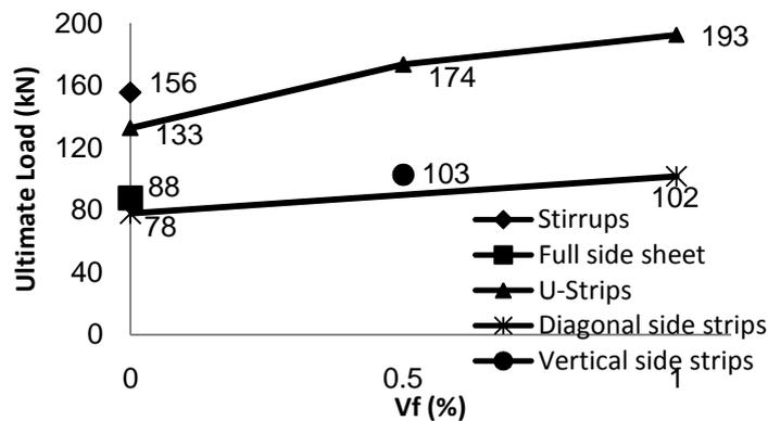
Figure (6): Effect of strengthening configurations and steel fiber content on ultimate loads.
