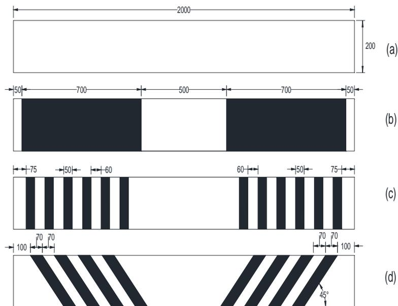
figure2. Shear strengthening configuration (All dimensions in mm).
