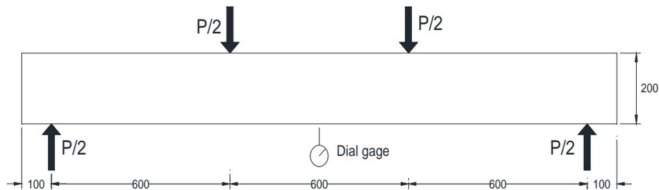
Figure4. Test Set-up (All dimensions in mm).
