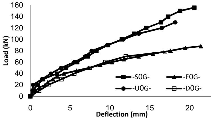
Figure (9): Load-deflection curves of GFRP reinforced beams with 0% steel fiber.
