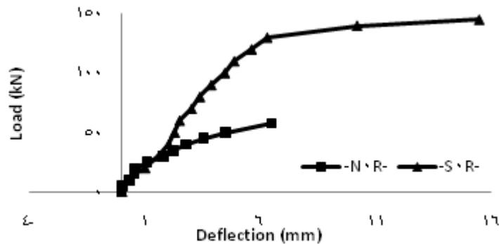
Figure (7): Load-deflection curves of steel reinforced beams.
