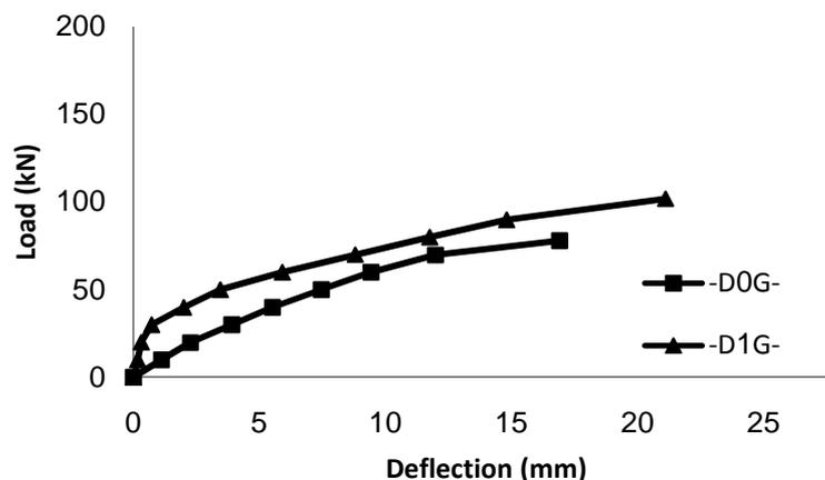
Figure (13): Load-deflection curves of GFRP reinforced beams strengthened by diagonal side strips.
