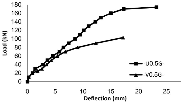
Figure (10): Load-deflection curves of GFRP reinforced beams with 0.5% steel fiber.
