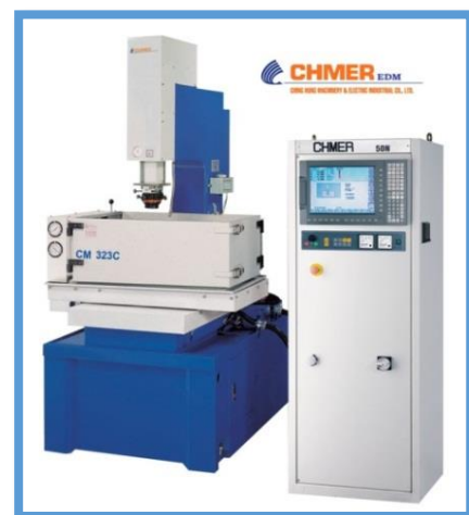
Figure 1: EDM Machine used for the experimentation Table 1: Machine specifications
