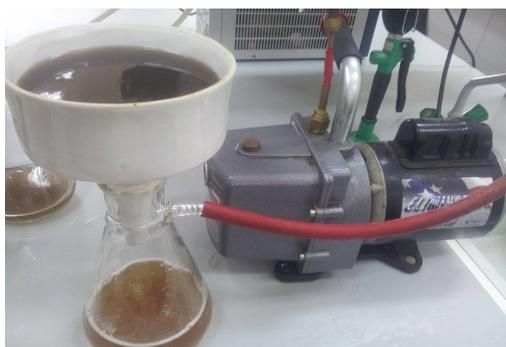
Fig. 2. Vacuum pump for washing and filtration process.
