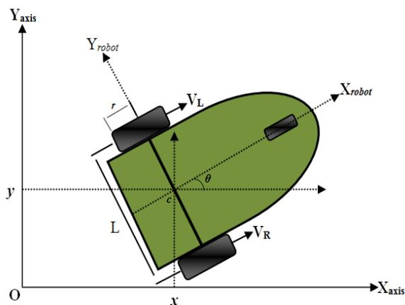
Fig. 1. Mobile robot Platform model.
