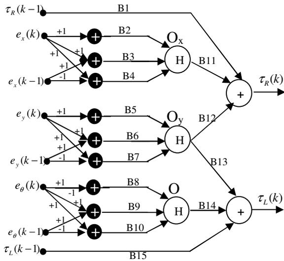
Fig. 3. The structure of nonlinear neural controller [3 and 4].
