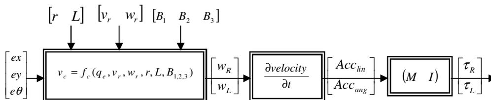
Fig. 4. The nonlinear back stepping controller structure [10].
