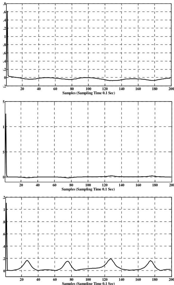
**Fig. 13.** Pose error of the mobile robot: a) error in X-axis; b) error in Y-axis; c) orientation error.
