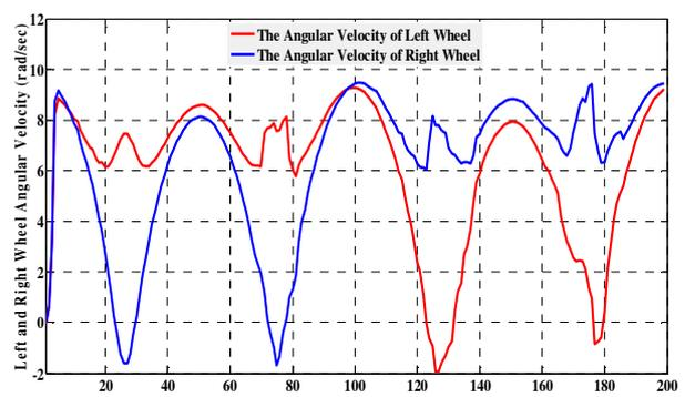
Fig. 11. Angular Velocities of the left and right wheels for nonlinear neural controller.
