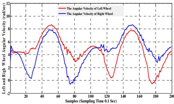
**Fig. 12.** Angular Velocities of the left and right wheels for nonlinear back-stepping controller.
