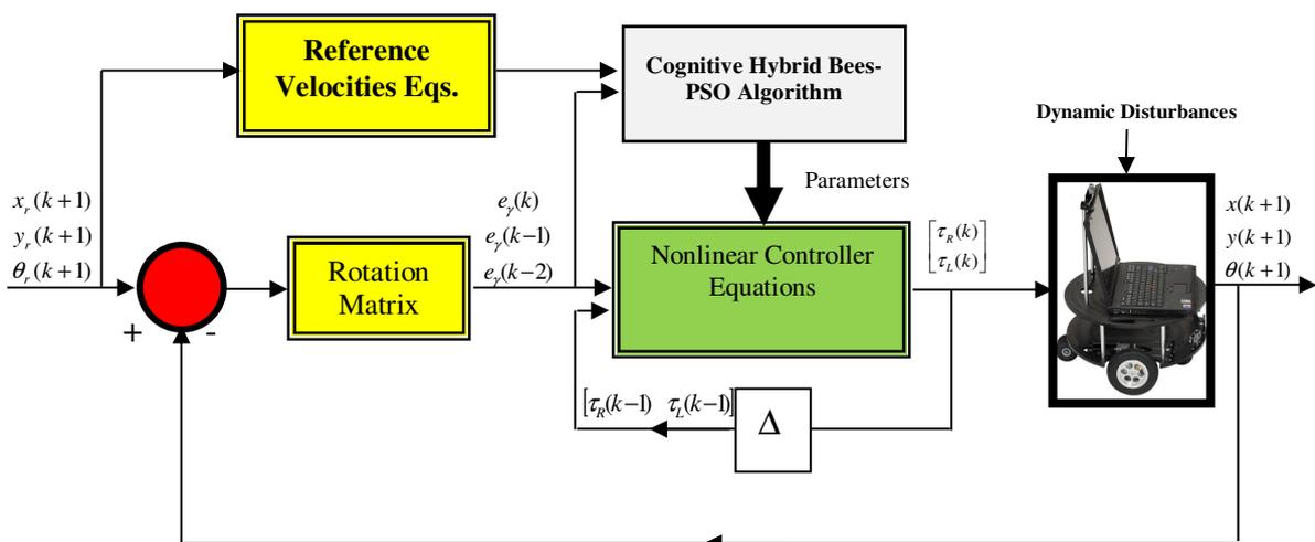
Fig. 2. The proposed structure of nonlinear trajectory tracking controllers for mobile robot.
