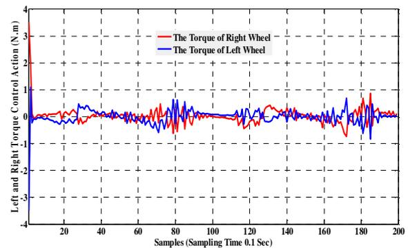
Fig. 10. Torque control action for nonlinear back-stepping controller.
