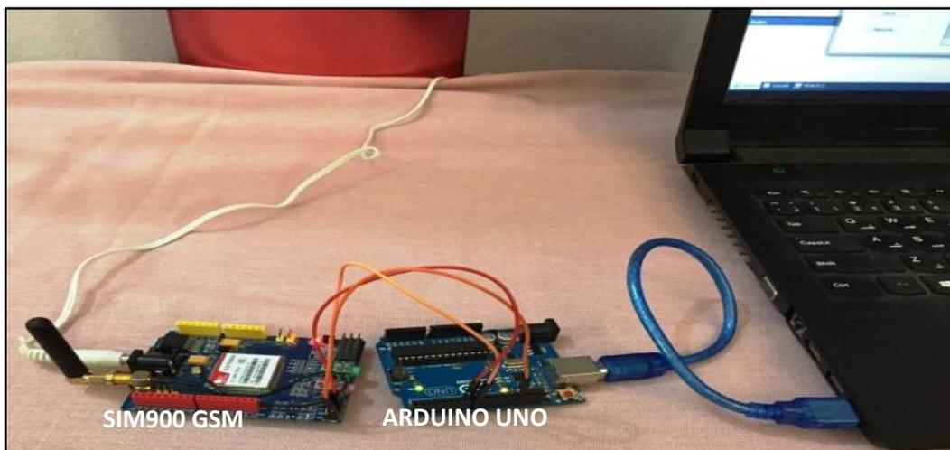
**Fig 7 : Connection of Arduino and GSM shield**
