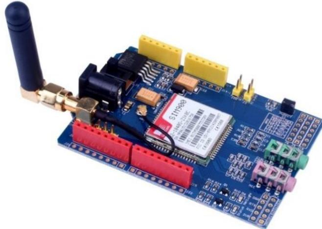
**Fig 2 : SIM 900 GSM Shield (Zatin *et.al.*, 2012).**
