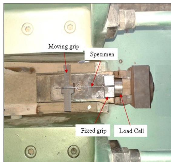
Fig. 3 Impact Tensile Gripping Mechanism
