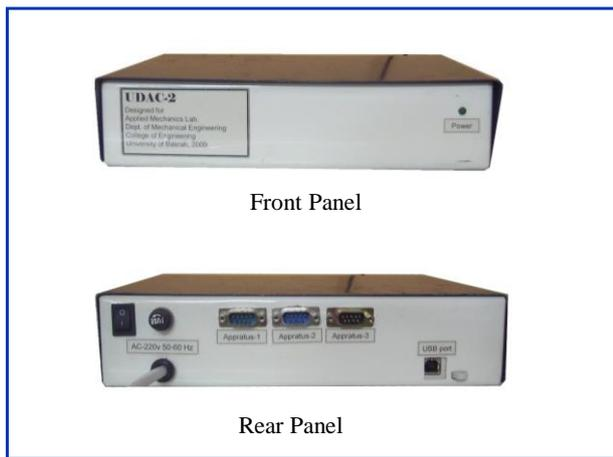
Fig. 4 The Interfacing Device UDAC-2.
