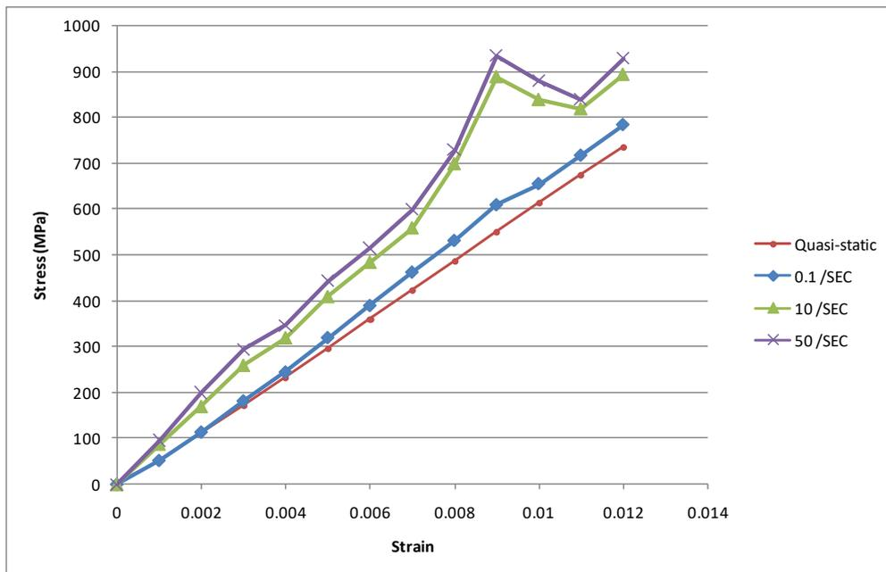
Fig. Stress-Strain Curves at Different Strain Rates. 7
