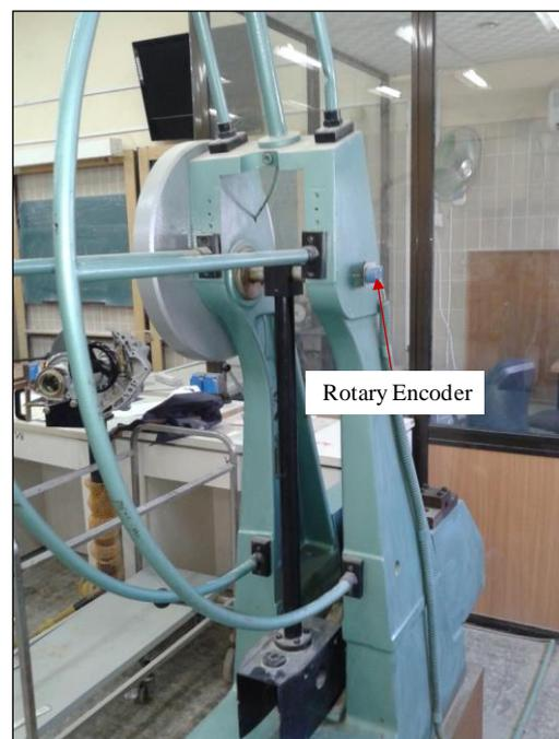
Fig. 2 Impact Testing Apparatus
