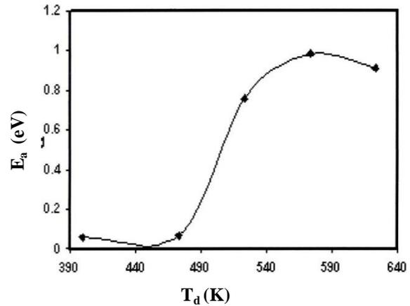
**Figure 2. Variation of  $E_a$  with  $T_d$  for CdS thin films with different diffusion temperature**
