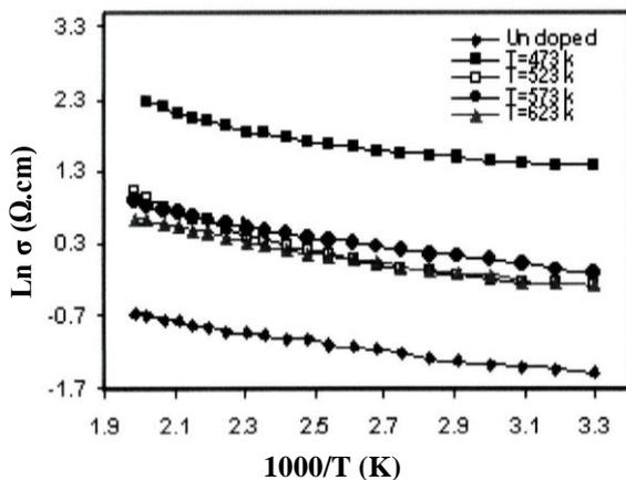
**Figure 1. Variation of the  $\ln\sigma$  with  $1000/T$  for CdS thin films with different diffusion temperature**
