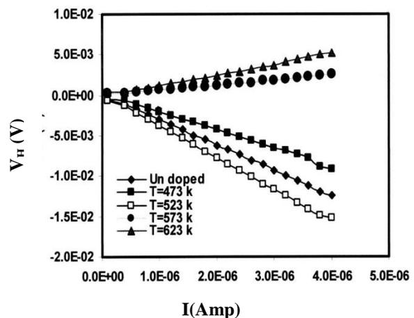
**Figure 3. Hall measurements for CdS thin films with different diffusion temperature**
