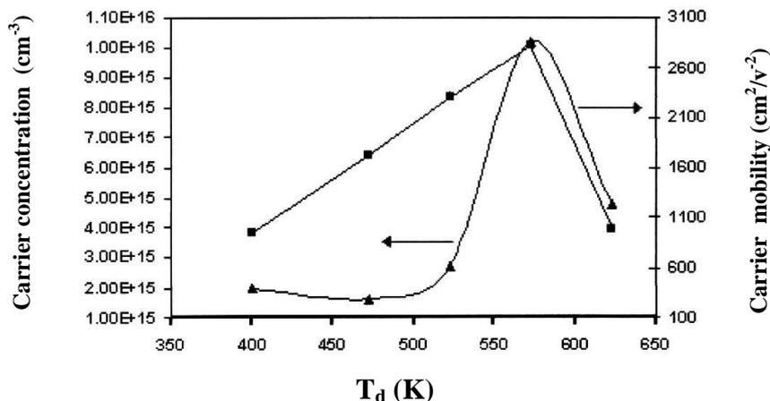
Figure 4. Variation of the concentration and mobility for CdS thin films with different diffusion temperature
