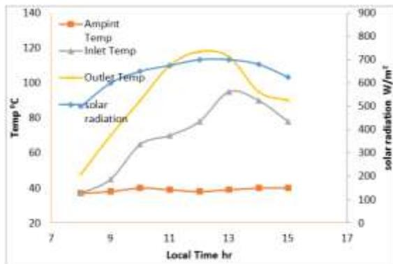
Figure (7) Show the solar radiation and temperature with time
