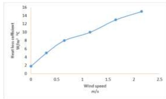
Figure (8) Show heat loss coefficient with variation wind speed
