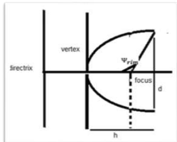
Figure (2) parabola
