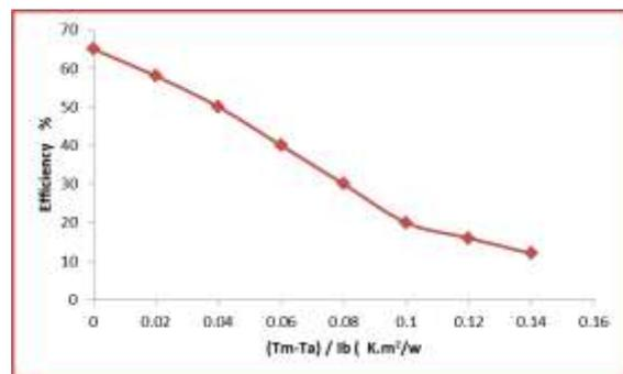
Figure (9) Show variation of efficiency with work temperature
