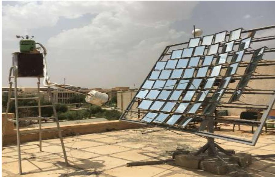
Figure (2) Show the fabricated solar dish array system.
