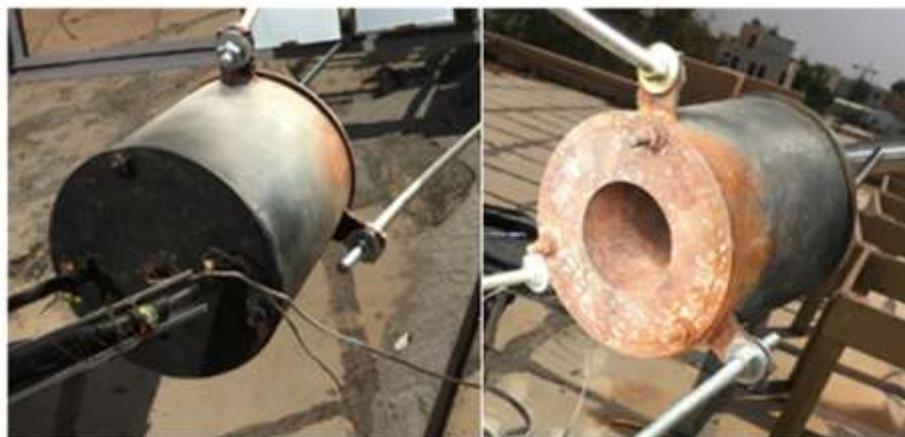
Figure (5) Show the front and back of the receiver (boiler) face and piping
