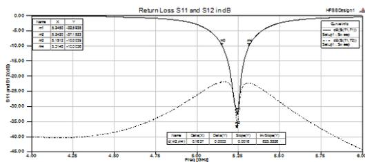
Fig. (8) Return loss  $S_{11}$  and decoupling  $S_{12}$  scattering matrix
