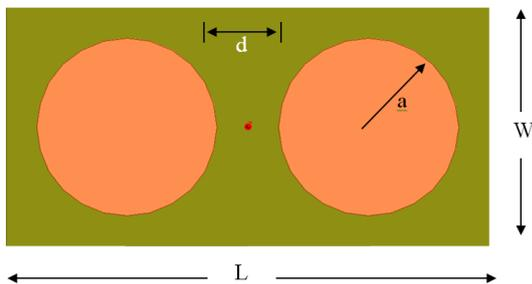
Fig. (3) Array antenna of two elements
