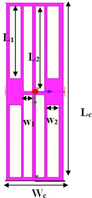
Fig. (6) Dimensions of the decoupling cell
