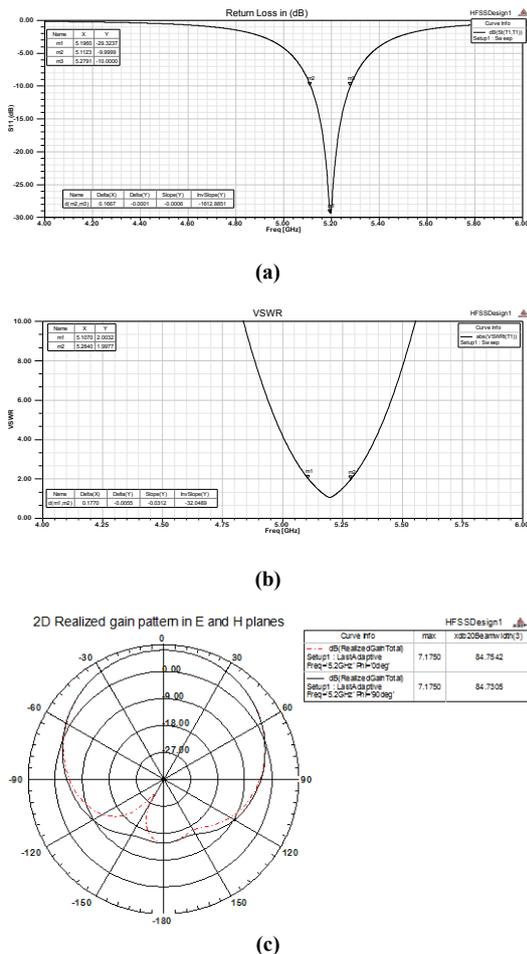
Fig. (2) Primary results (a)  $S_{11}$ , (b) VSWR, and (c) Realized gain
