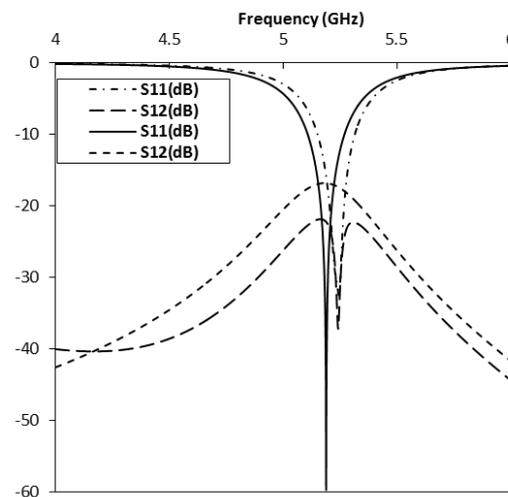
Fig. (10) Comparison between graphs of  $S_{11}$  and  $S_{12}$  with (red solid and dashed curves) and without (black solid and dashed curves) decoupling cell
