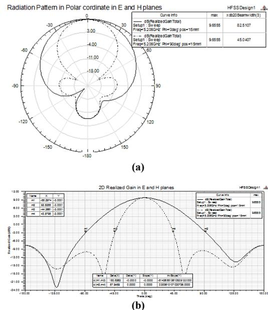
Fig. (5) Radiation pattern (realized gain) of array antenna (a) polar coordinate and (b) rectangular coordinate
