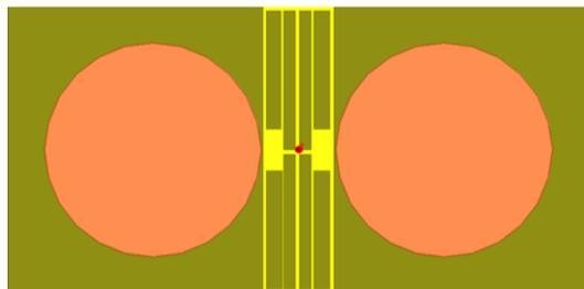
Fig. (7) Array antenna with decoupling cell
