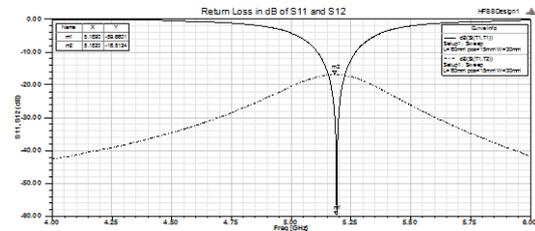
Fig. (4) Return loss  $S_{11}$  and coupling factor  $S_{12}$  of array antenna
