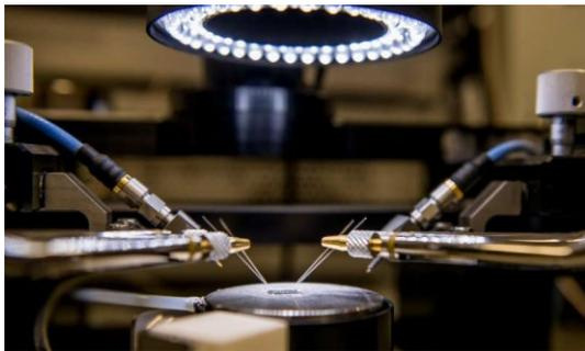
Electrophysical characteristics of the detector were tested on a probe station. Credit: Evgeniy Pelevin/MIPT
