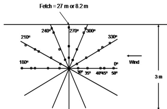
Fig. (2) Plan view of experimental arrangement showing the locations of the centers of the illuminated areas.
