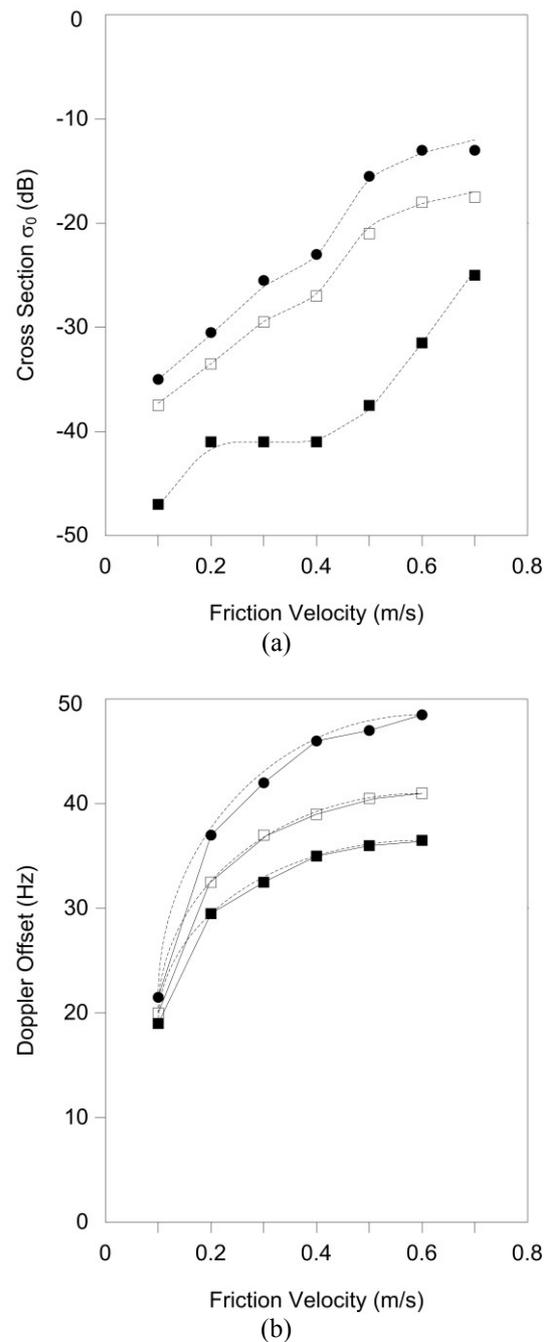
Fig. (6) Cross sections and Doppler offsets measured with 2 cm wavelength incident radiation at a 50° incidence angle looking upwind with a fetch of 6.5 m. The lines indicate the following: lower dashed = HH, bound waves move at their own phase speed; dotted = HH, bound waves move at the phase speed of the first harmonic of the dominant wave; dash-dotted = HH, solid = VV, upper dashed = sonar, all assuming bound waves move at the dominant wave phase speed
