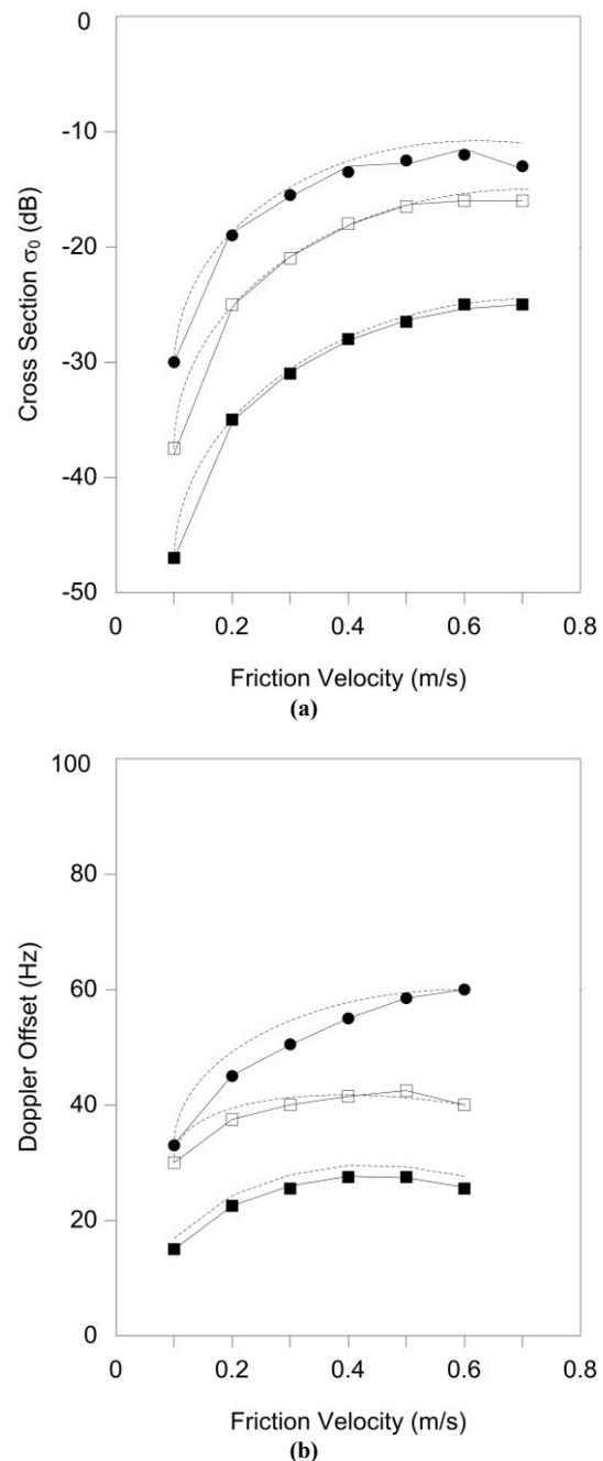
Fig. (3) (a) 2 cm cross sections versus friction velocity, (b) 2 cm Doppler offsets versus friction velocity. Data were taken at with 2 cm wavelength radiation and a  $50^\circ$  incidence angle with both radar and sonar directed upwind. Symbols: + = sonar, x = radar HH, o = radar VV. Data at 5 m fetch (solid lines) were collected in 2005 in the UW wind-wave tank; those at 6.5 m (dotted lines) and 25.5 m fetches (dashed lines) were collected in 2011 in the large wind-wave tank
