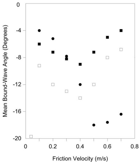
Fig. (7) Mean bound wave slopes measured in these experiments and in previous experiments. Symbols indicate the following fetches:  $\square$  = 6.5 to 7.8m, this experiment;  $\blacksquare$  = 25.3 to 26.6 m, this experiment;  $\bullet$  = 5.0 m, Plant et al, 1999b; points = 14.3 m, Plant et al., 1999a. All values were derived from microwave and acoustic measurements except the points, which came from direct measurements using a laser slope gauge
