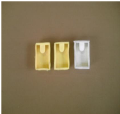
Fig(4-a) : polysiloxane molds polysiloxane
