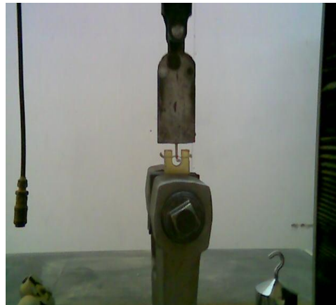
Fig(4-d): U-shaped specimen under tensile tester
