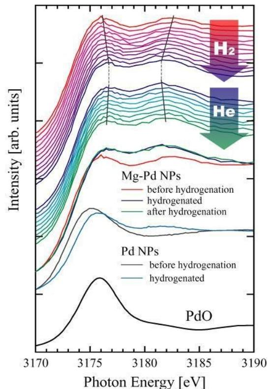
Fig. (5) The change of the Pd L<sub>3</sub>-edge NEXAFS for the Mg-Pd nanoparticles during the hydro-/dehydrogenation. The spectra of the Mg-Pd nanoparticles before hydrogenation or hydrogenated are also shown. The spectrum of the PdO is shown as the standard
