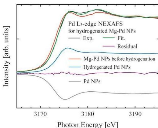
Fig. (6) The simulation of the Pd L<sub>3</sub>-edge NEXAFS of the Mg-Pd nanoparticles after hydrogenation by the linear combination fitting
