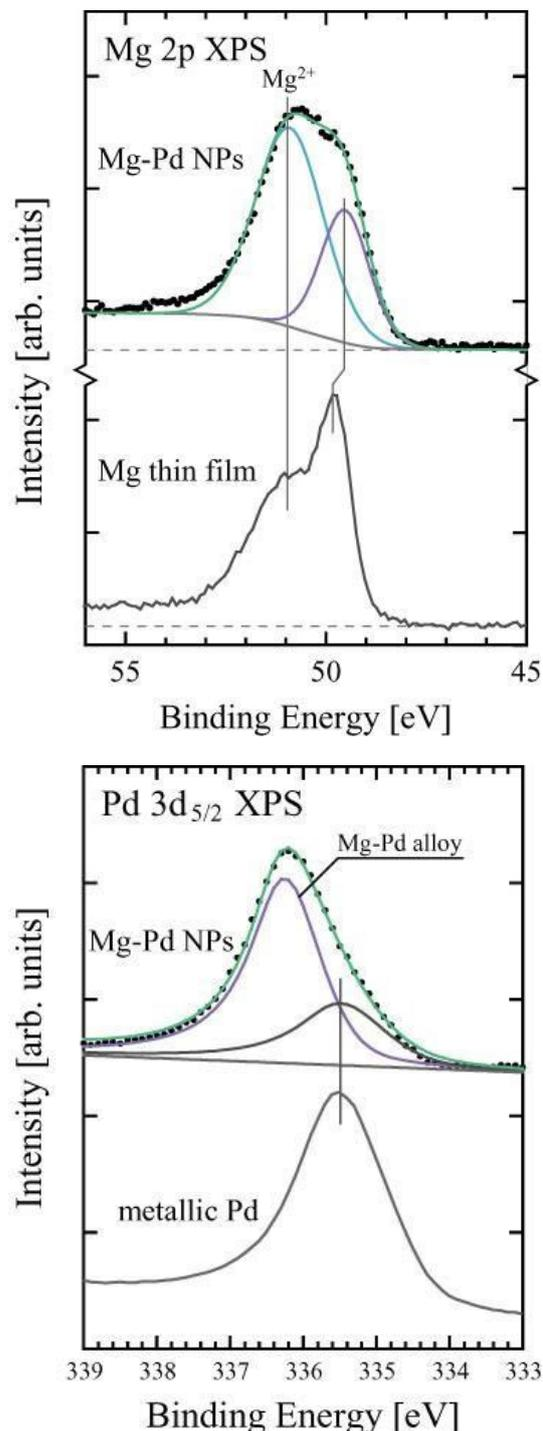
Fig. (3) The XPS spectra for the Mg 2p and Pd  $3d_{5/2}$  core electrons of the Mg-Pd nanoparticles. The XPS spectra of the metallic Mg and Pd are shown as the standard spectra. The Mg 2p spectrum of the Mg-Pd nanoparticles has been obtained by subtraction of Pd 4p spectrum
