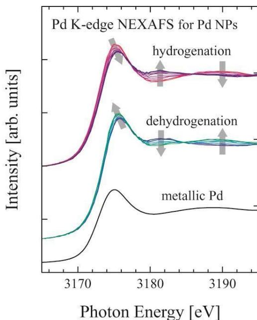
Fig. (4) The change of the Pd L<sub>3</sub>-edge NEXAFS for the Pd nanoparticles during the hydro-/dehydrogenation. The spectrum of the metallic Pd is shown as the standard
