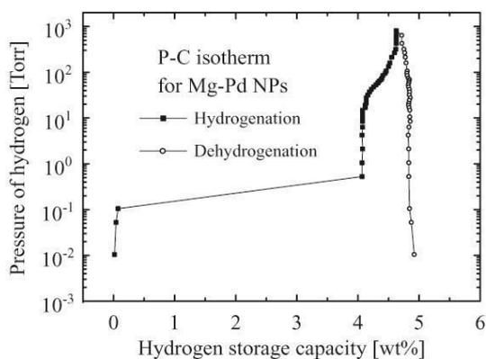
Fig. (1) The P-C isotherms for the hydro-/dehydrogenation of the Mg-Pd nanoparticles at 303K
