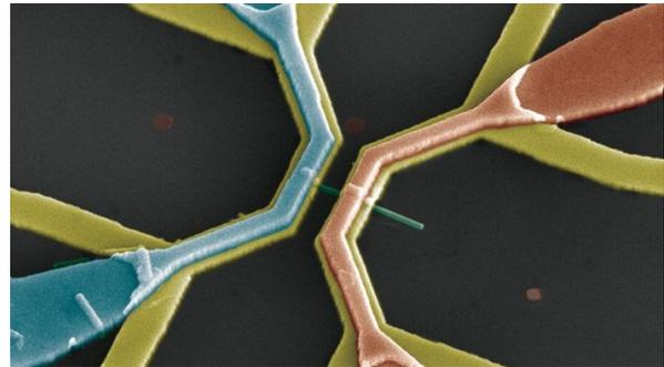
A nanoscale heat engine, shown in false colour, includes a nanowire (green), metallic elements (yellow), a heater (red) and a cold element (blue). Credit: M. Josefsson et al./Nature Nanotechnol
