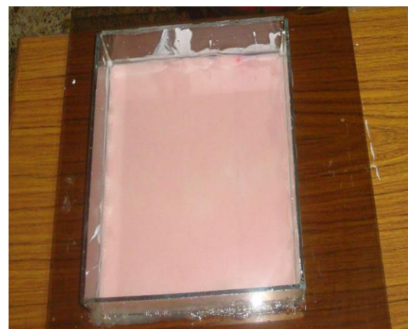
Figure 3: Casting of Composite Specimens in Glass Mould.
