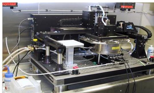
Figure2.  $\text{CH}_4$  gas sensor measurements setting.
