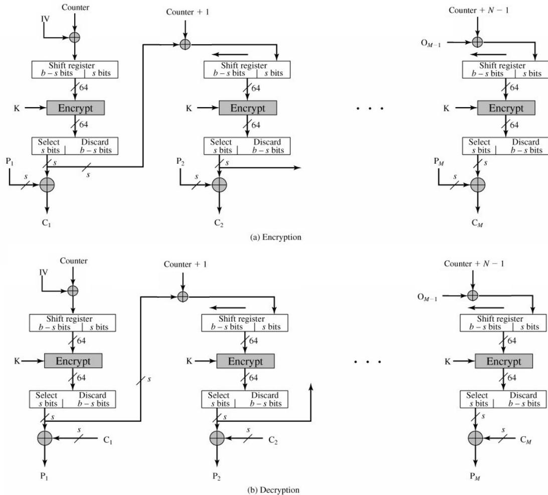
Figure.4: s-bit Counter Output Feedback (COFB) Mode
