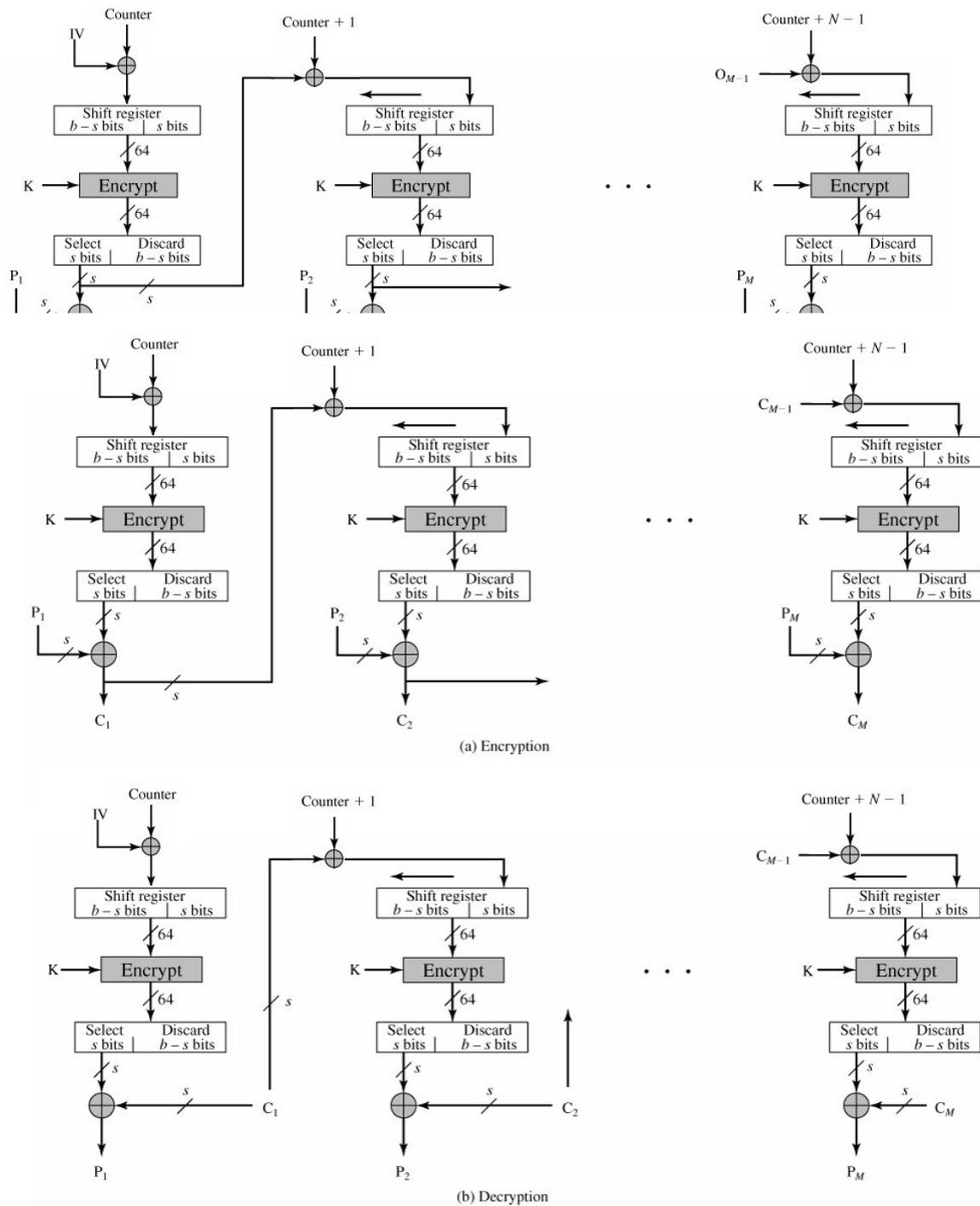
Figure.3: s-bit Counter Cipher Feedback (CCFB) Mode
