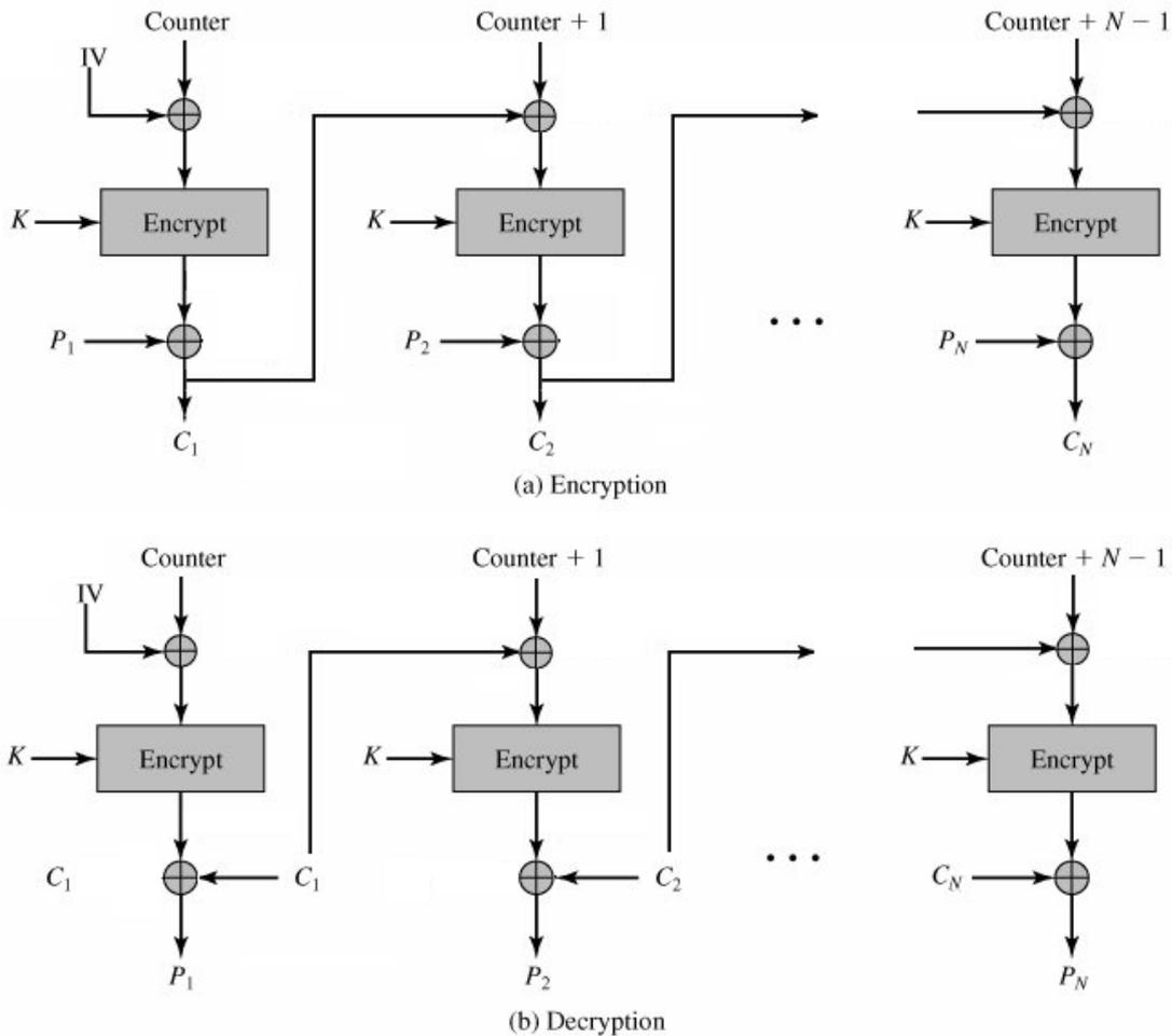
Figure.2: Counter Cipher Block Chaining (CCBC) Mode
