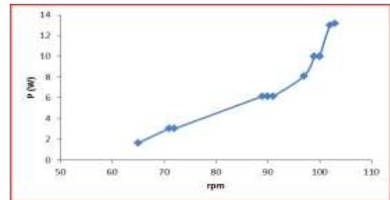
Fig. 8. Relation between power and rpm.
