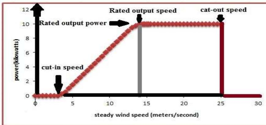
Fig. 1. wind speed with power output [14].
