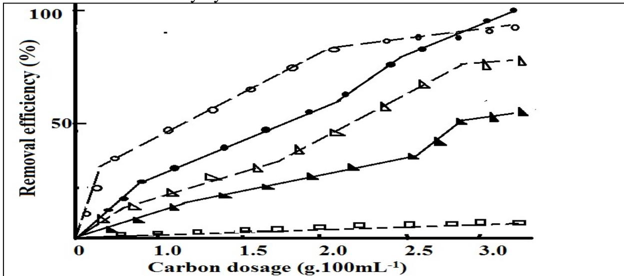
Fig.1. The efficient removal of COD by the five types of activated carbons. Steam treated (o), acid-treated (Δ), base-treated (▲), heat-treated (□) and commercial activated carbon (●).
