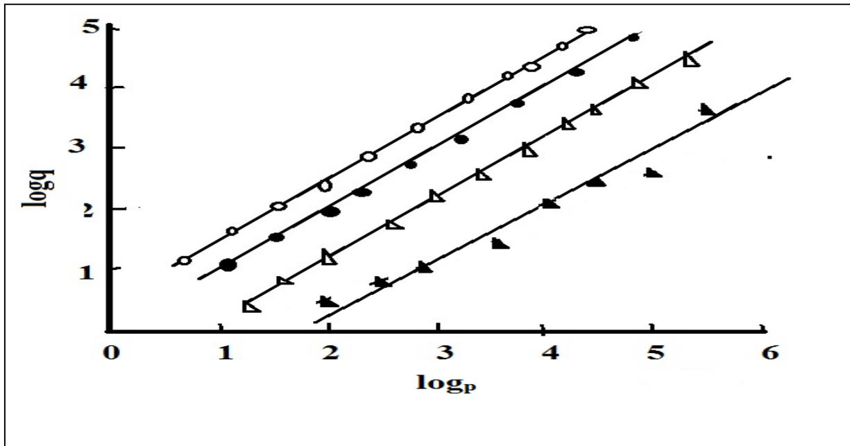
Fig.2. Freundlich plots for the COD adsorption onto the activated carbon. Steam treated (o), acid-treated ( $\Delta$ ), base-treated ( $\blacktriangle$ ), and commercial activated carbon ( $\bullet$ ).
