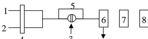
Fig.1. Chemical reaction manifold used for the flow injection chemiluminescence determination of adrenaline hydrochloride.
