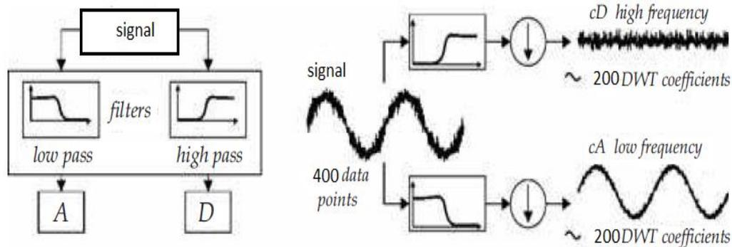
**Fig. 1. Decomposition of a signal by wavelet analysis**
