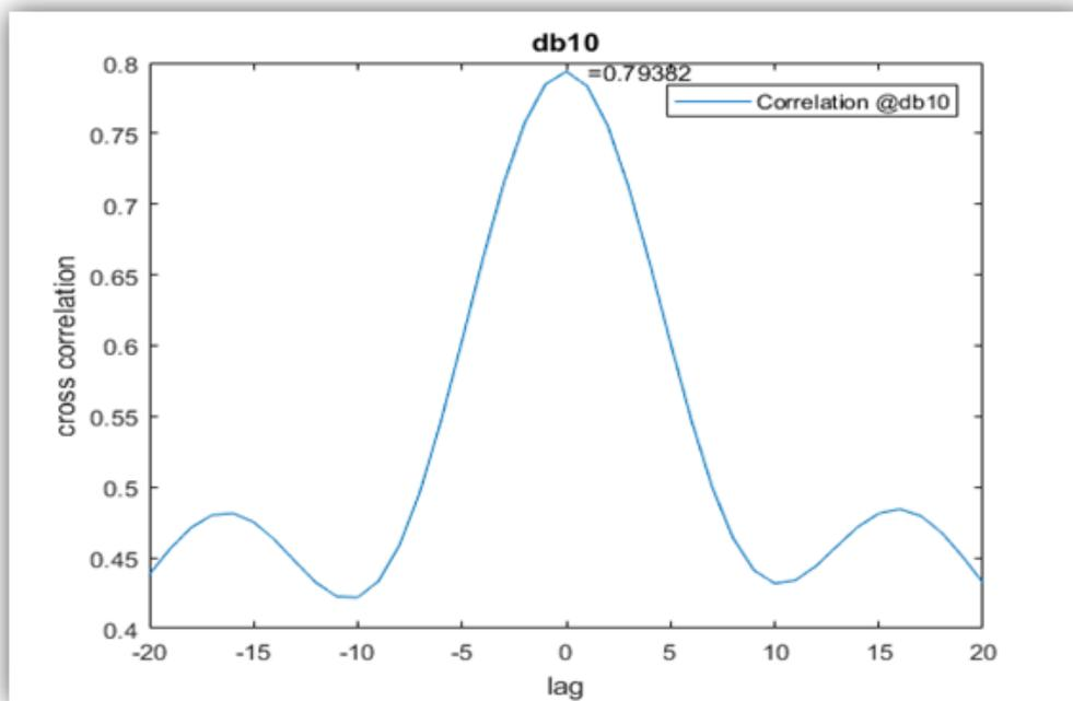
**Fig. 3.** Graphs of the cross-correlation functions for noise cancellation using the Daubechies wavelet (the value the zero point is 0.79382) of the tenth order
