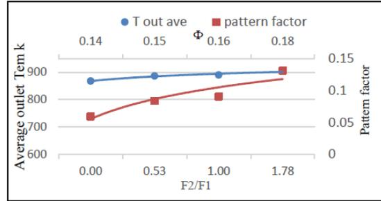
**Figure 8, pattern factor and average outlet temperature with EGR ratio 20%.**
