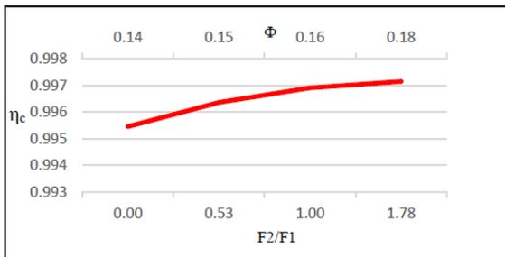
**Figure 9, combustion efficiency for loaded turbine 95 cm H<sub>2</sub>O compressor outlet pressure EGR ratio 20%.**
