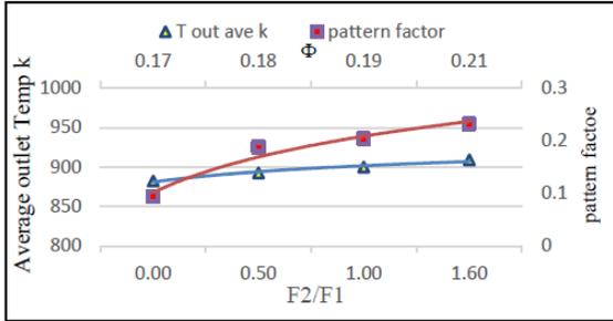
**Figure 7, pattern factor and average outlet temperature without EGR effects.**
