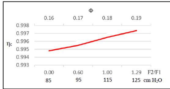
Figure 17, Combustion efficiency for loaded turbine with difference compressor outlet pressure.
