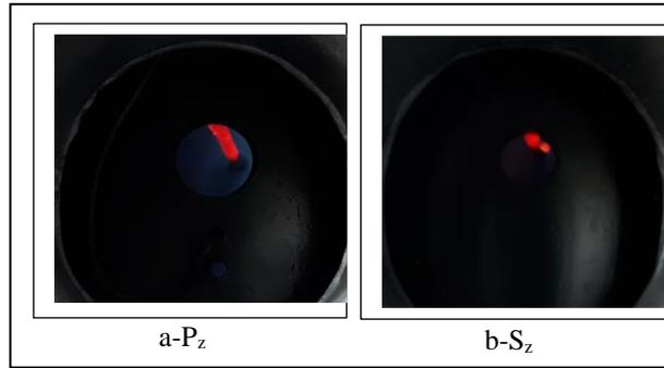
**Figure 4 a and b Photographs of flame in primary zone and secondary zone respectively**
