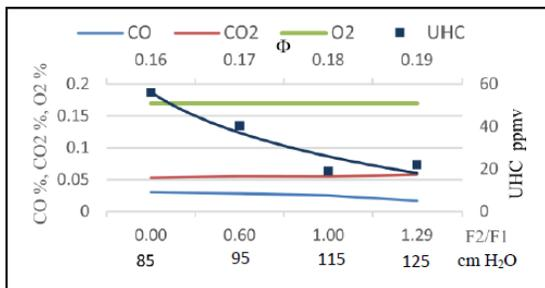
Figure 18, Emission gases with equivalence ratio for loaded turbine and with EGR effects.
