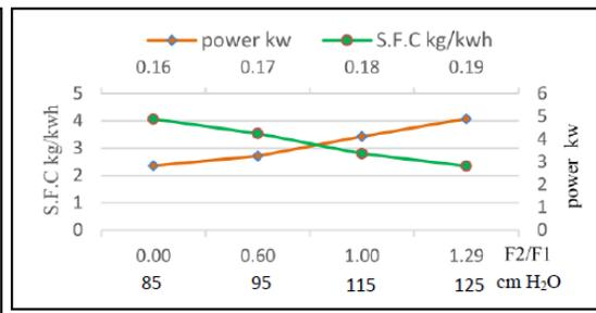
Figure 19, Power and S.F.C for loaded turbine with difference compressor outlet pressure
