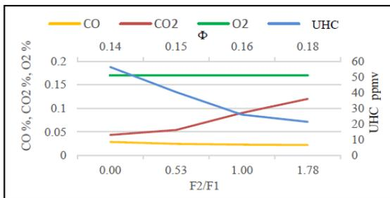
**Figure 11, emission gases for loaded turbine 95 cm compressor outlet pressure EGR ratio 20%.**
