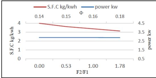
**Figure 13, power and S.F.C loaded turbine 95 cm compressor outlet pressure EGR ratio 20%.**
