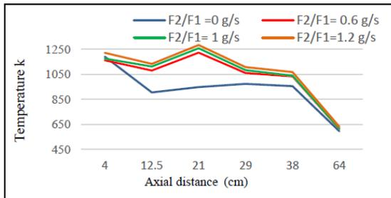
**Figure 5, temperature profile along the combustor for loaded turbine 95 cm H<sub>2</sub>O compressor outlet pressure with EGR ratio**
