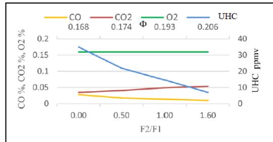
**Figure 12, emission gases for loaded turbine 80 cm compressor outlet pressure EGR ratio 25%.**
