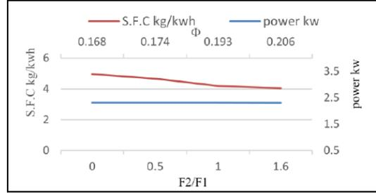
**Figure 14, power and S.F.C loaded turbine 80 cm compressor outlet pressure EGR ratio 25 %.**
