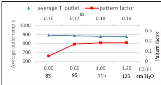
Figure 16, Pattern factor and average outlet temperature loaded turbine with difference compressor outlet pressure.
