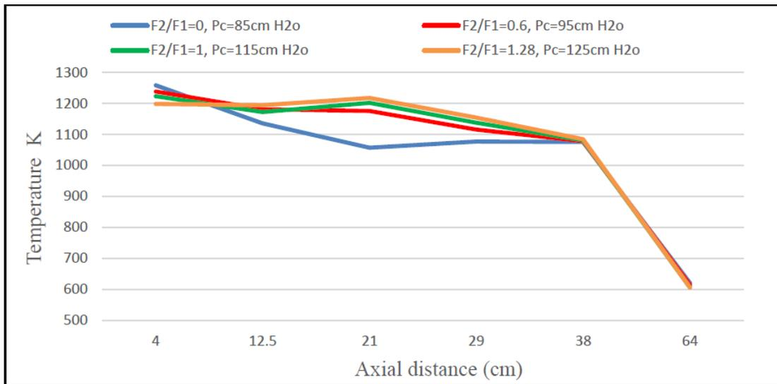
**Figure: 15 temperature profile along the centerline of the with EGR effects loaded turbine with difference compressor outlet pressure.**
