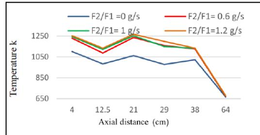
**Figure 6, temperature profile along the center line of the combustor for 60 cm compressor outlet pressure.**
