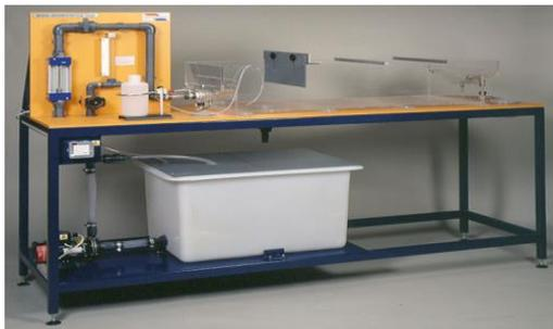
**Figure 1:** The Armfield Model Sedimentation Tank
