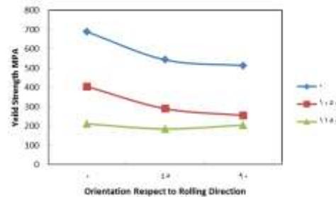
**Figure 4:** effects of anisotropy on yield strength of stainless steel samples under different annealing temperatures
