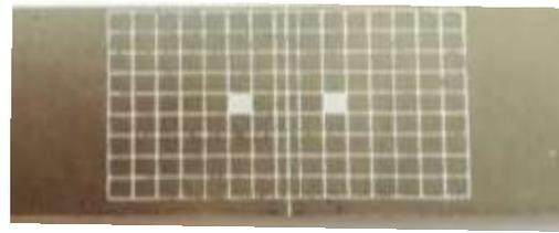
**Figure 2:** grid for strains and displacements measurement
