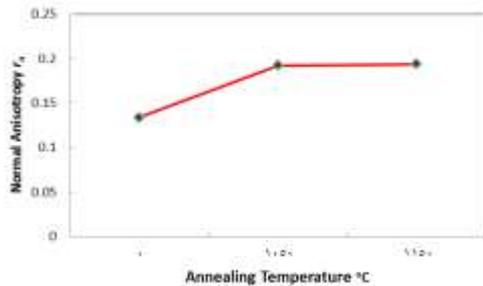
**Figure 5:** effects of annealing temperature on normal anisotropy
