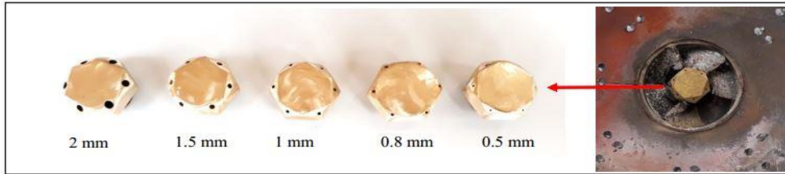
Figure: 3. Swirler with the variable Main injector holes size.
