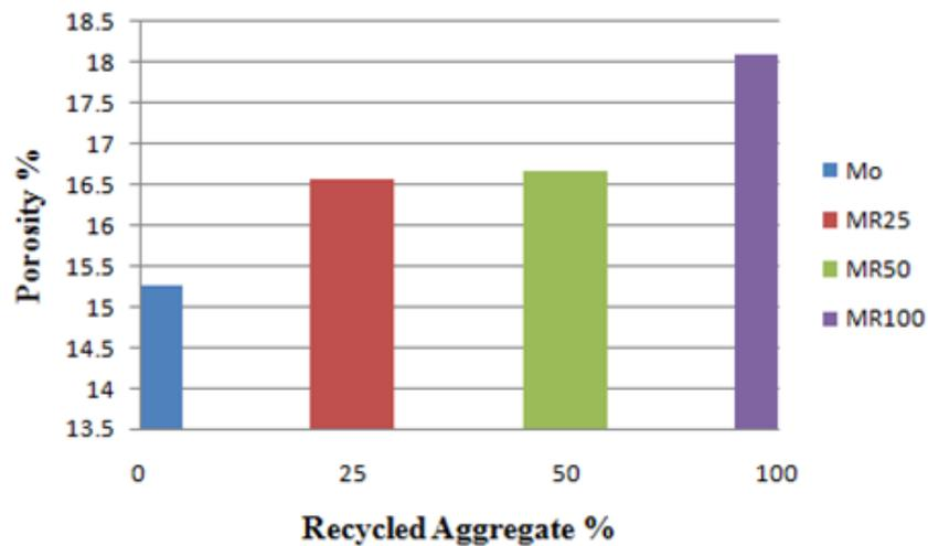
Figure 3. Percentage of porosity of recycled cement mortar samples.
