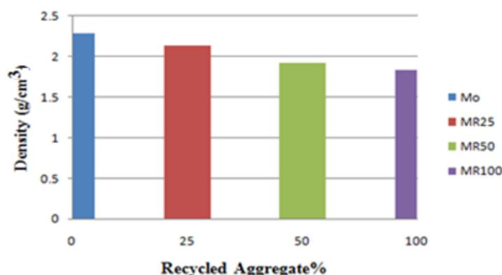
Figure 1. Apparent density of recycled cement mortar
