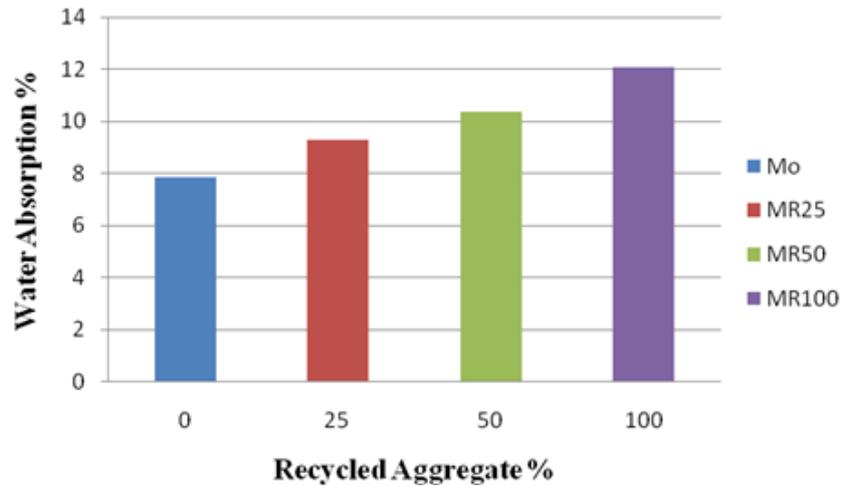
Figure 2. Percentage of water absorption of recycled cement mortar samples.
