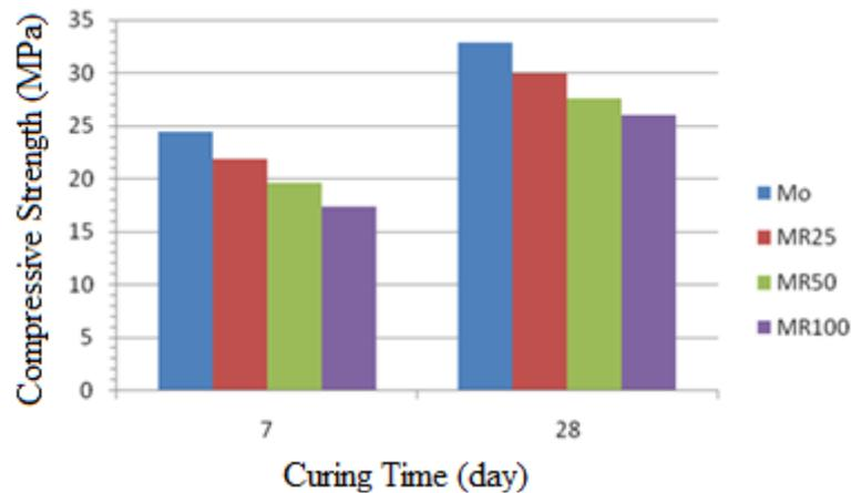
Figure 4. Compressive strength for cement mortar samples at 7 and 28 day
