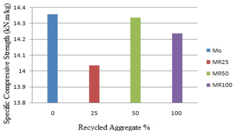
Figure 5. Specific Compressive Strength for prepared cement mortar samples at 28 day.
